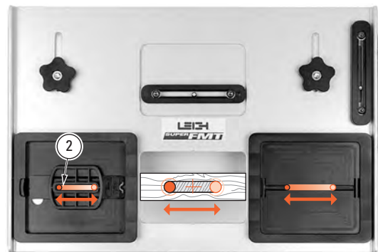
3-25 Mortises are routed with the guide pin running in the inside mortise slot of the guide ②. Always rout the mortise slightly deeper than the tenon length. Note: In most constructions, only one tenon and perhaps two mortises need to be cross marked and sighted. Please read all of the procedural chapters to gain the utmost efficiency from your Super FMT. ■
