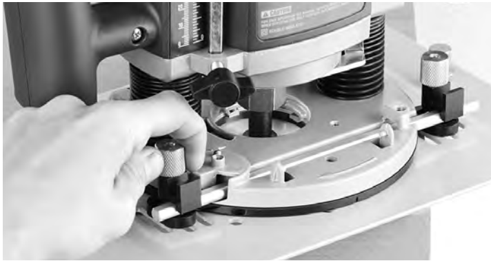
2-17 Turn down the four brass knobs until there is only very slight and even pressure on each end of both rods. Leave the sliding stops in the outer position.
