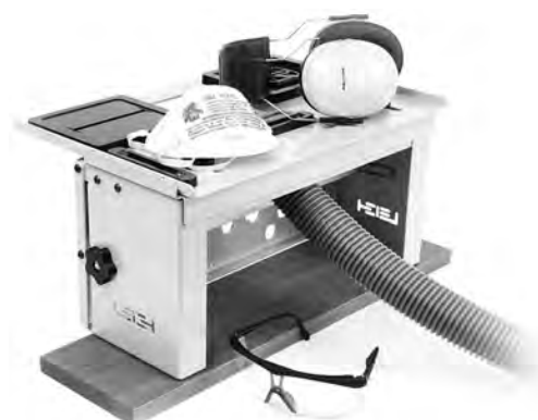
3-27 Always wear approved safety glasses and hearing protection. Protect yourself from harmful dust by wearing a face mask. We highly recommend you acquire and use the optional Leigh Super FMT Vacuum Attachment. Connect your shop vacuum or dust collection system directly to the vacuum box.
