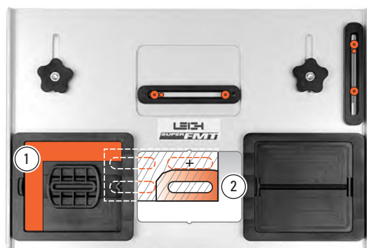
5-29 With practice, it is fairly easy to avoid routing into an adjoining tenon, however, we do recommend that beginners use a simple “L”-shaped shop-made guard to prevent this ①. Use 1/4" [6mm] MDF or plywood and allow a 3/16" [5mm] gap between the guide and guard. Rout the front right tenon ②.
