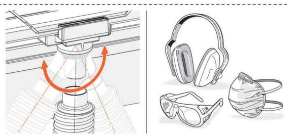
**21 Safety** The improved swivel joint nozzle on the VRS provides highly efficient dust and chips collection but like all shop dust collection systems, it can't be 100% effective. When routing, always wear approved protective eye, ear and breathing gear.
