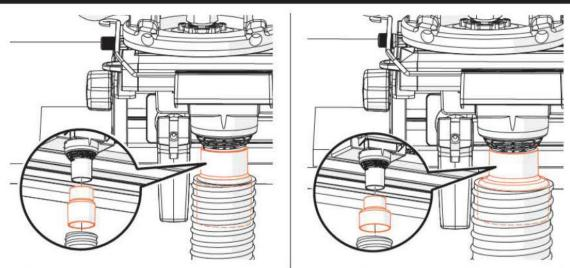
**19** Attach the shop vacuum hose directly to the collector nozzle or use one of the two hose adaptors supplied. Try keeping the front clamps vertical and turned away from the hose adaptor to allow maximal router travel.
