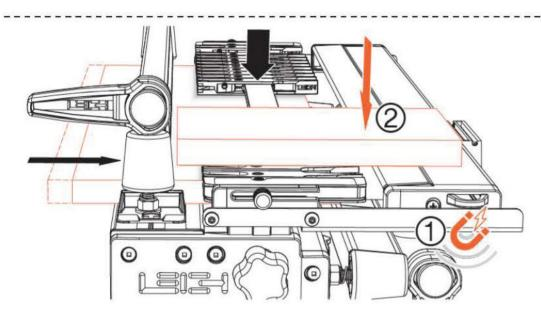
**14** Install the spacer board and jig finger assembly on the jig and lower it onto the support board. Install the VRS onto the steel brackets ①. It attaches magnetically. Lay a piece of flat board ② on the finger assembly, extending out over the top of the VRS extrusion.
