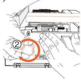
**10** Loosen the support bracket knobs and while holding the board down flush on the finger assembly, raise one steel bracket until the **peak** ① on top of the VRS extrusion touches the underside of the board. Now tighten the knob at that end ②. Repeat at other end. **Double-check and readjust both ends as needed until the finger assembly is level with the VRS extrusion peak.**
