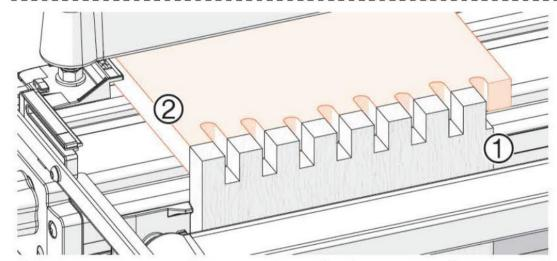
**20** For maximum efficiency, always back up vertically mounted workpieces ① with a backer board ②. This not only prevents chips and dust exiting the rear of the board, it also aids in preventing tear out from the rear of the workpiece.
