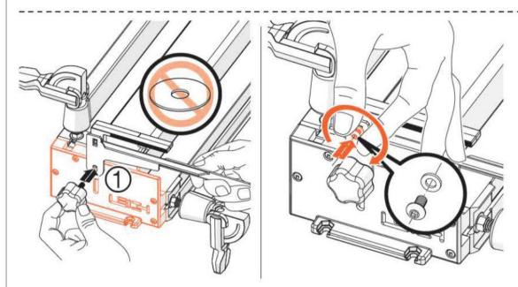
**8** If the end housings look like this ①, it's a D4R Pro, D4R or late model D4 jig, and the nylon washers **should not be used**. Install the two 10-24 button head screws and washers, one at each end, finger tight only.
