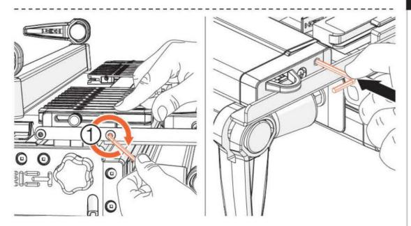
**16** Now firmly tighten the other two button head screws ①. The hex key stows in the right hand end of the VRS.
