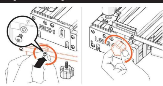
**13** Attach the pair of steel VRS support brackets to the cast finger support brackets (with the horizontal surfaces inwards) using the four 10-24 button head screws and washers, **but just finger tighten only.**
