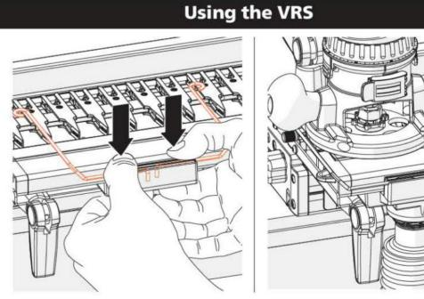
17 Install the two router follower rails by placing the wire ends into the selected holes as far as possible; then using thumb and index finger, squeeze and **snap** the arm down into the end of the slot. Position the wire brackets to allow routing of the workpiece outer edges. Efficient waste collection does not require centering the router bit in the collector.
