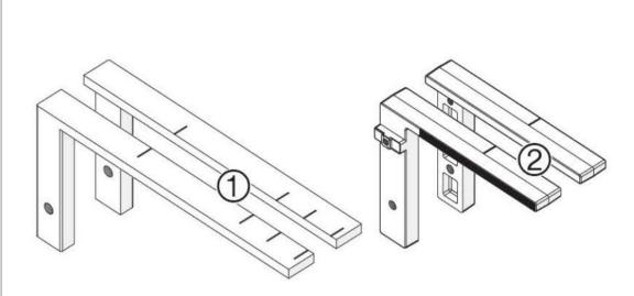
**6** D4R Pro, D4R, D4, 24"(610mm) D3, D1258R and D1258 owners With the exception of the D4R Pro, first remove the long support brackets ① from your jig (or short brackets from your D1258/R, not shown). Then, install the **new** short brackets ② included with the VRSD24. **D4R Pro Jig owners: The new brackets** ets are identical to those supplied with your jig. Keep as spares.
