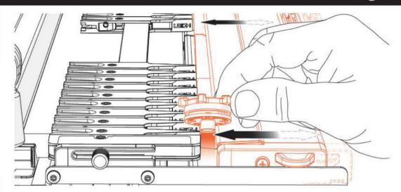
**18** Adjust the VRS forward/backwards to create a gap between the extrusion and the jig guide fingers (or template), that is slightly greater than the guide bushing's diameter used.
