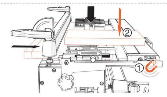
**9** Install the spacer board and jig finger assembly on the jig and lower it onto the support board. Install the VRS onto the steel brackets ①. It attaches magnetically. Lay a piece of flat board ② on the finger assembly, extending out over the top of the VRS extrusion.
