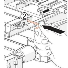
11 Now firmly tighten the two button head screws ①. The hex key stows in the right hand end of the VRS ②. After installation, when raising and lowering the combined VRS and finger assembly, always take the weight at the inner end of the brackets ③, not at the VRS ends. Note: The VRS height may need to be reset when using Isoloc or Box Joint Templates.
