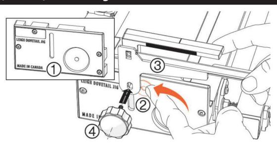
**7** If the end housings of your jig look like this ①, slide one of the nylon washers ② between the steel bracket ③ and the end housing, and then thread the bracket knob ④ back in. Repeat this step on the opposite end of the jig.
