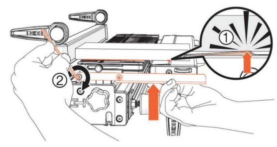
**15** Starting on one end, raise one steel bracket until the VRS extrusion's **peak** ① touches the underside of the board. Now tighten only the rear screw with the provided hex key ②. Repeat step for opposite end. **Double-check and readjust both ends as needed until finger assembly is level with VRS extrusion peak.**
