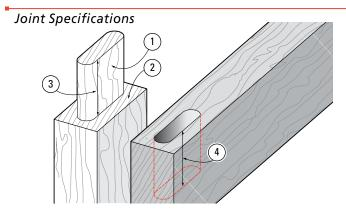
**A1-1 Joint Terminology** The tenon sides are the "Cheeks" ①. The tenon shoulders are called (luckily) the "Shoulders" ②. Unfortunately, references to dimensions of mortises and tenons do not share matching terminology, so... Long or short tenons ③ fit into deep or shallow mortises ④.
