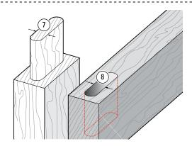
**A1-3** Thick or thin tenons 7 fit into wide or narrow mortises 8.
