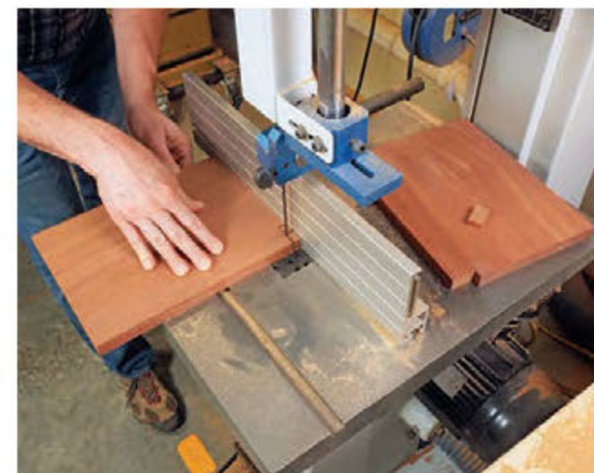
Both the top panels and shelves of the outer units will require notches along their back inside corners in order to fit around the back legs of the center unit. Make these cuts with a band saw, jigsaw or backsaw.
