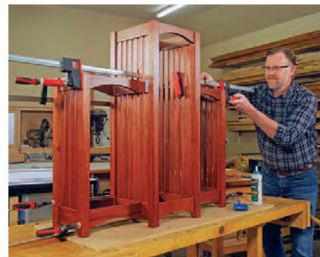
Check the fit of all of the outer units' components before opening a glue bottle. If all the joints close properly, round up a bunch of clamps and assemble the outer and center units with glue.
