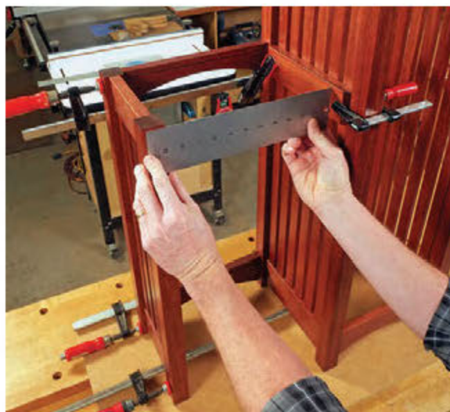
Sand, stain and topcoat the arched rails, then go ahead and bring the center unit together with glue and clamps.
