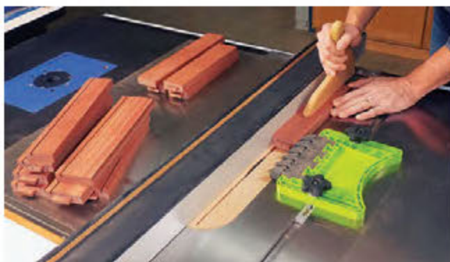
Rockler's Table Top Fastener hardware requires that one end fits into a saw kerf. Cut these kerfs 5/16" deep and 7/16" in from one edge of each front and back rail on what will be the inside face of the parts.
