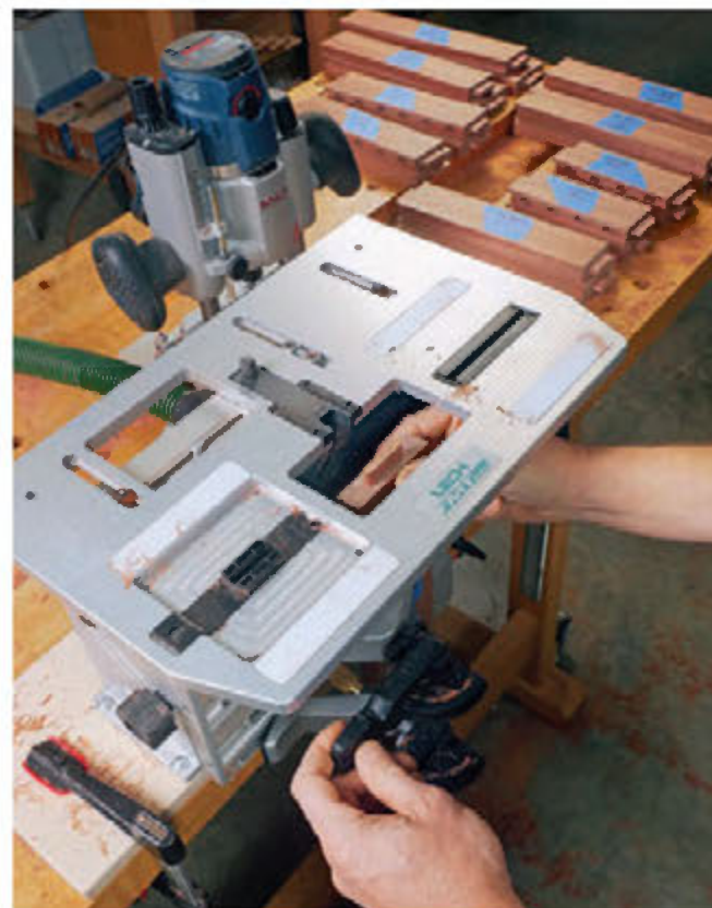
The same plastic template used for mortising also sets the jig for cutting a matching tenon. Two cam-activated clamps on the FMT hold workpieces vertically for this second milling operation with a spiral bit.
