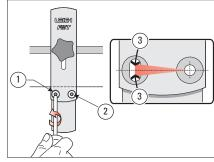
loosen the 'pivot' screw ① and the right hand 'lock' screw ② with the FMT hex driver. Adjust the angle ③. Tighten the screws and rout test joints to establish the correct setting by trial and error. Once locked in this position it should never require adjustment when used with that same router.
