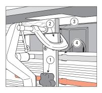
①, the fence may be inverted with the short end up in the bit opening ②. A suitable small clamp is used to hold the mortise piece against the face of the short fence ③ which is perfectly flush with the clamp plate face ④. When routing mortises at the end of a board, always move the table as far as possible left or right to minimize the length of unsupported workpiece.
