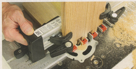
Sturdy handles on the ends of the fence assembly make the jig easy to control. Cam-style clamps hold workpieces and backup boards securely.
