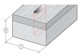
A1-11 Maximum Mortise Board Width and Thickness for Mortising to Center
