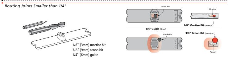
4-36 Example: 1/8" (3mm) Mortise & Tenon Joints with a 1/4" (6mm) Guide Using the two bits and guide shown above, you can rout a 1/8" (3mm) mortise and tenon. The resulting joint is 1/8" (3mm) smaller than the 1/4" guide size. Note: Any two bit diameters that add up to twice the guide size will produce a joint size of the smaller bit.
