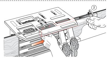
**4-30** Sight the second mortise by moving the mortise piece (**not the table**) and set the second stop block ②. Rout any number of successive (unmarked) mortises without removing the router from the table.
