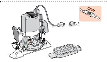
**4-7** Unplug the router. Insert the selected guide in the guide recess and the matching diameter bit to the router. Note: See Appendix I for Guide and Bit Selection.
