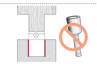
**4-25** Generally we have found the best fit differential to be 0.005"[0,13mm] "loose". Basically, the dry joint should "push" together fairly easily, but not fall apart under its own weight. If a mallet is needed, it's too tight.
