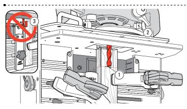
**4-11** Plunge the router so the tip of the bit is level with the pencil mark of the tenon shoulder and lock the plunge ①. Set the plunge depth stop rod to its stop ②. *Generally, tenons are routed in one depth setting, it is not necessary to make multiple passes at different depths of cut.* A WARNING: Never rout tenons with the sidestop fence in the inverted position ③.
