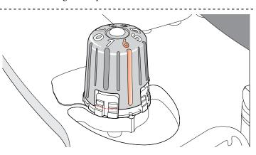
**4-26** Once you have established the guide pin setting for a specific bit/guide combination, record the setting.
