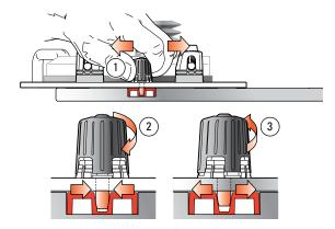
**4-9** Adjust the right hand guide pin. Grip right hand pin knob and move sub-base back and forth to feel the "free play" of the pin across the slot width ①. Turn knob down ¼ of a turn at a time, to feel the "play" diminish ②. When the "play" stops, turn knob up ½ of a turn until the slightest play can be felt ③. The router/sub-base should slide freely left to right. If right pin is a little "sticky", turn it up a bit more.
