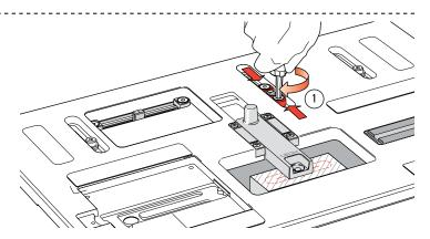
**4-6** Unlock the two **BFB** front/back limit stops. Move both so they touch the Stop Post and tighten both stops ①. This prevents front-to-back movement of the table when later sighting the mortise. Retract the sight.
