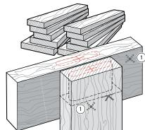
**4-27 Production Procedures** When routing frame joints it is only necessary to mark and sight a single tenon and perhaps two mortises. Once the side stop fence or outriggers are set and the table sighted for one joint, any number of similar joints may be routed without marking and without removing the router from the jig. We recommend marking the finished face which goes against the clamp plate (shown here from operator view) ①.
