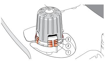
**4-10** Check that the left hand knob is two turns up. From this setting the actual fit setting will be established by trial and error and the result recorded for each guide/bit combination. Note: The "steps" in the height "washer" indicate numbers of "turns up"; one turn ① two turns ② three turns ③ Never turn the knobs up more than 3½ turns in use.
