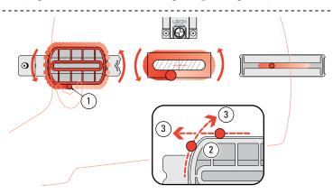
**4-14** Routing counter-clockwise, run the guide pin around the tenon guide surface. Make sure the pin contacts the entire outer surface ①. In these first test cuts, check the tenon for a completely smooth cut before removing the piece from the jig. Until you are confident with this procedure, we recommend as a final clean-up, you run the guide pin "off" of each guide "corner" ② in both directions ③.
