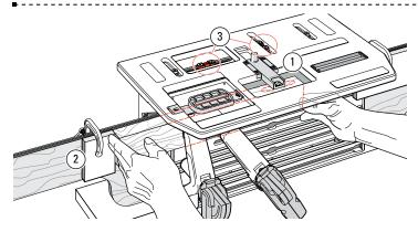
**4-29 Mortises:** Sight one mortise ① and set a stop block at the end of the mortise board ②. Set **ab LR** limit stops and **BFB** limit stops to prevent unintentional table movement ③.
