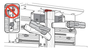
**4-4** Clamp the tenon piece with the end edge **lightly touching the underside of the sight**. Its side edge should touch the previously set side stop fence, with the marked side toward the clamp plate.
