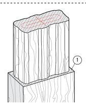
**4-13** Control the router firmly, the router is driven clockwise by the bit rotation. This first shallow climb cut will leave a small but clean shoulder ①.
