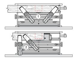
**4-15** Remove the router and tenon workpiece from the jig. Position the two clamps so the mortise piece can be positioned for secure holding. Clamp to either both sides of the vacuum box ① or to one side ②. Note: Leaving a "horn" on the ends of mortise pieces as in ① not only makes for easy clamping, it's good woodworking practice as the horns will be an aid in assembly gluing and clamping later.
