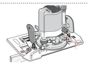
**4-17** Place the router/Sub-Base assembly on the jig, the left hand guide pin in the mortise slot part of the guide. Now raise the plunge stop rod slightly, say ½2-¼16"[1-1,5mm] to allow the mortise to be routed slightly deeper than the tenon to ensure perfect tenon shoulder flushness on the finished joint.
