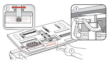
**4-16** Extend the sight. With the marked side of the mortise piece toward the clamp plate, either move the board left and right ① to align the cross with the sight and clamp in place; or clamp in place first and move the table to align the sight ②. Remember, you previously set the **BFB** limit stops to allow only left/right movement. For routing very small pieces ③, see 3-16.
