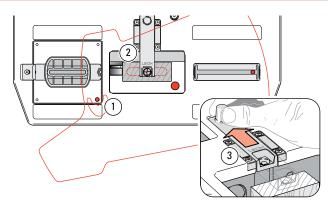
**4-28 Tenons** The router is "parked" with the guide pin in near front corner of recess ①. Extend sight and use only as a tenon stop ② when clamping successive (unmarked) tenon pieces against side stop. Retract sight ③ and rout any number of tenons without removing router. Note: If you forget to retract the sight, the Sub-Base will push it out of the way as you move it rearward, but we do not recommend this.
