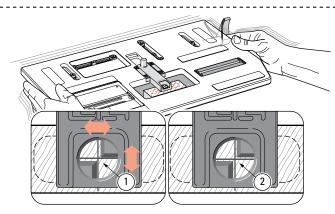
**4-5** Release the table clamp and move the table until the sight opening is positioned equally around the cross lines on the workpiece. Lock the table. Because the human eye excels at comparisons, differences as small as 0.004" can be perceived in the space between the edges of the line and the triangles as shown here ①. You can readily center the sight using slight table movements until the spaces appear the same ②.
