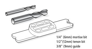
4-34 Example: 1/4" (6mm) Mortise & Tenon Joints with a 3/8" (9mm) Guide Using the two bits and guide shown above, you can rout a 1/4" (6mm) mortise and tenon. The resulting joint is 1/8" (3mm) smaller than the 3/8" (9mm) guide size. Note: Any two bit diameters that add up to twice the guide size will produce a joint size of the smaller bit.
