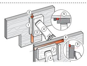
**4-40** To hold very small workpieces ②, make up a rabbeted holder ③ with the rabbet slightly shallower than the workpiece thickness, leaving a gap at ⑤ and ⑨. i.e. For Tenons: Side stop ① Tenon Piece ② Holder ③ Clamp ④ Gap ⑤. For Mortises: Mortise Piece ⑥, Holder ⑦, Clamp ④, Gap ⑨.
