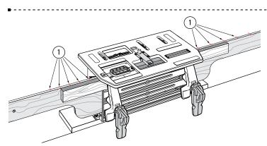
**4-31** Successive mortises in "ladder" type construction are quick to rout. Mark all mortises on only one piece (only one needs a front-to-back mark!). Sight the first mortise (cross) to set the table and mark the top of one outrigger in line with the workpiece end. Table locked, move the workpiece, sighting each successive mortise line, marking the outrigger(s). To rout, align the unmarked board ends with the outrigger marks ①. ■
