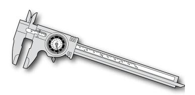
**4-24** If you have a dial or digital calliper (every shop should have one) you can literally measure the tenon and mortise and adjust accordingly.
