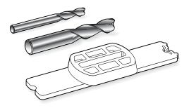
**4-33 Two Bit Combination** If you want to rout many 1/4"[6mm] mortises and tenons, the tenons can be routed much more quickly with a 1/2"[12mm] bit\*. The Guide and Bit Selection charts in Appendix I show how different bit combinations can crank out such extraordinary joints just as quickly and precisely as larger ones, and with adjustable joint tightness.
