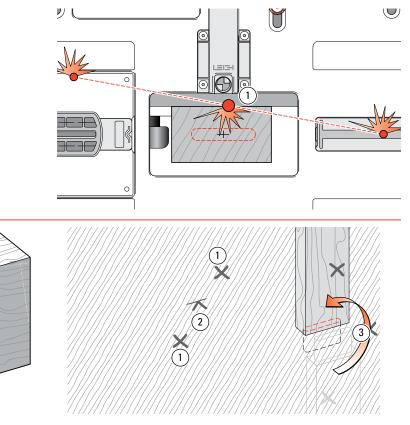
**4-1** Let's make a plain single mortise and tenon. Using a fine pencil, mark a cross at the center of the required tenon and mortise. The cross lines along and across the axis lines of the joint must be at 90° to each other. Mark the mortise several inches[10cm] or so away from the end.
