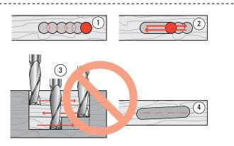
**4-18** The best way to rout mortises (parallel to workpiece) is plunge full depth, slightly overlapping holes ①, then clean out left-right-left at full depth of cut ②. Do not rout left-right-left at progressively greater depths without plunging holes ③ ... the bit's rotation will pull the bit off the intended mortise line with each pass ④ and the mortise may not be parallel to the workpiece.
