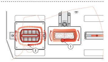
**4-12 Read all of the next 3 instructions before routing.** With guide pin in near side of guide recess, switch on router power and with firm control, move it in until the bit lightly touches the tenon workpiece. Very carefully, with bit very lightly engaging the wood surface, "climb rout" clockwise around tenon piece ①. Maintain very light bit contact. Do not run guide pin on guide yet ②.
