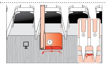
**15-1 Through Dovetail Pins** With the straight bit, carefully climb-rout from right to left. Make sure you control the router firmly when climb routing.
