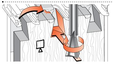
**15-7 Dovetail Tails Tearout** With the dovetail bit, most tearout occurs at the top left exit of the cut.
