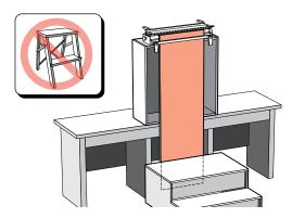
**15-13 General Hints** For routing long vertical boards it may be necessary to build a jig stand to mount securely on your bench. Make the stand and bench height combination sufficient to accept the board length you have in mind. The jig stand should be bolted securely to the bench. Build a stable platform to stand on as in the illustration. **Do not use a set of steps; they're too unstable.**
