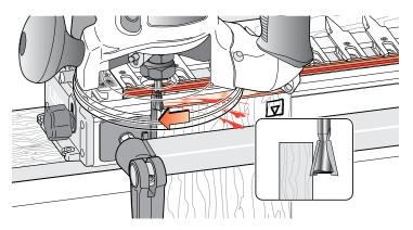
**15-12** On face cuts, whether using a straight bit or a dovetail bit, climb routing or back routing will leave a clean edge; but great caution must be exercised in controlling the router's movement from right to left, as the bit rotation pulls the router in that direction anyway.
