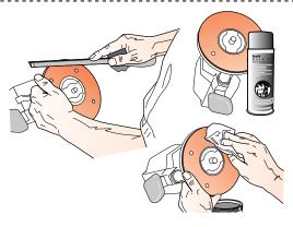
**15-16** Some router bases have sharp edges on the outside and inside corners. A slight chamfer of the edges with a fine file or sandpaper block will ease router movement on the jig.
