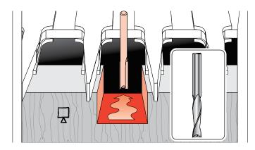
**15-5** Rout away the rest of the waste. Note: Spiral up-cut straight bits (inset) generally rout more smoothly than the two-flute carbide-tipped bits. If you want to try them, you should be aware that while the high-speed steel bits take a better edge, they are much less durable than the more costly solid carbide type (Leigh bits 170 HSS or 170C solid carbide).
