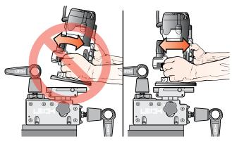
**5-5** Do not tilt the router on the jig.Keep the router flat on the jig assembly.*Note: The optional Leigh VRS attachment prevents router tilting.*
