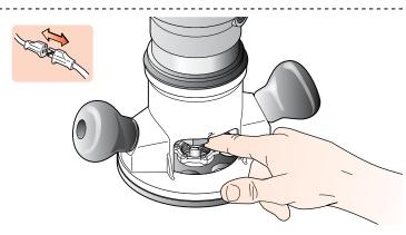
**5-4** Always disconnect the power source from the router when fitting bits or guidebushes, or making adjustments.
