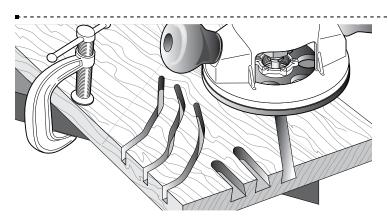
**5-9** If you have never used your router before, be sure to follow the router manufacturer's instructions for its use. Make plenty of simple open-face practice cuts *without a guidebush* before you try to use the router on the Leigh jig. You must, of course, always use a guidebush when routing on the Leigh Jig. ■
