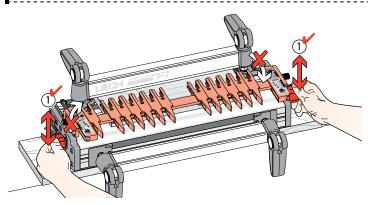
**2-1** Practice with the finger assembly height adjustment. Loosen the support bracket knobs and hold them firmly. Raise and lower the assembly evenly, **keeping it level** ①, and tighten the knobs to lock it at various heights. **Do not raise or lower only one end of the finger assembly.**
