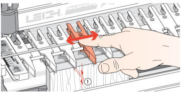
**2-2** To practice adjusting the guidefingers, put a board in the front clamp. Always raise the finger assembly slightly, approximately ½16"[2mm] above the spacer board and/or workpiece ①. This is essential to allow the guidefingers to move freely on the guidefinger bar and ensures that the fingers will be level and flush when locked up. Move the guidefingers by pushing on the middle to slide them along the guidefinger bar.
