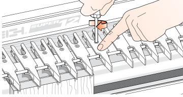
**2-5** Always tighten unused guidefingers before routing, as router vibration may cause loose screws and finger lock parts to fall out and be lost.
