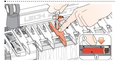
**2-3** Loosen about half the guidefingers and practice unlocking, moving, positioning and re-locking them. Always press on the center of the guidefinger when tightening the screws. This ensures that the small pads ① on the inside of the finger contact the face of the finger bar ② and keeps all the fingers level.
