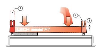
**1-21** For all but the wider workpieces, you need only operate the clamp on the workpiece end of the jig to release the board ①. For narrower boards, the clamp at the free end ② should be just tight enough to bow the clamp bar about  $\frac{1}{16}$ "[2mm] ③.
