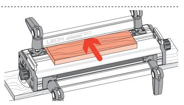
**1-12** Make up a spacer board. This will be used to support the finger assembly in all front-clamping vertical board modes. Use MDF or plywood for flatness and stability. We suggest <sup>3</sup>/<sub>4</sub>"x 6"[20x150mm], in lengths of 11"[280mm] for Super12, 17"[430mm] for Super18, and 23"[600mm] for Super24. Note: Thickness of spacer board has no relationship to thickness of vertical board being routed. Clamp board in rear of jig.
