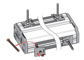
**1-2** Insert the two front clamp T-bolts through the jig body holes. Make sure the bolt's "T" is between the extrusion ribs. Place a front side stop and steel washer over each bolt but only finger-tighten the front nuts; you will need to index these to the rear stops later.
