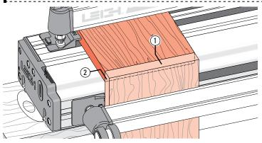
**1-9** Now loosen the front clamp and position the front board so its top end edge is perfectly flush and level with the top face of the horizontal board ① and, both boards left edges are also perfectly flush ②. Tighten the clamp.
