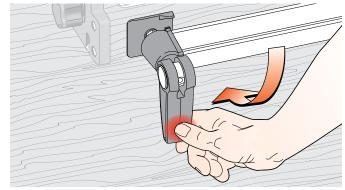
**1-20** A smooth, firm action is enough to engage the clamp. Rule of thumb: If you can't throw the lever by pressing the end of it firmly with your thumb, reduce the tension. Firm thumb pressure is about right. A few minutes of trial and error will help you feel the right clamp tension.
