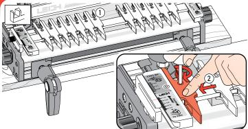
**1-16** With the finger assembly in PTD Pins mode ①, move the outer end guidefingers to touch the scale block and lock in position ②. *Note: the outer end guidefingers are used for router support only.* When guidefingers are loosened, the finger assembly should easily slide on the support brackets. If not, apply a little candle wax to the mating surfaces.
