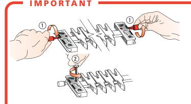
**1-13** Before using the jig, the scales must be set into position on the finger assembly. Install the two thumbscrews a few turns into the scales ①. Loosen the scale lock screw ② at each end by one turn only.
