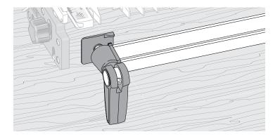
**1-19 The Jig Clamps** Use a piece of flat, even-thickness wood to familiarize yourself with the jig cam clamps. You will operate the cam-action speed clamps every time you use the jig, so get used to the feel of the clamps first. **Do not force the cam-action speed-clamp**. It has great leverage, and excessive force may damage the workpiece or the jig.
