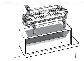
**1-23** To gain height for a more comfortable working position or for routing longer boards, mount the jig to a box that can be bolted securely to a bench. *See also 15-13.*
