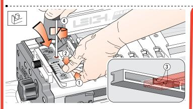
1-15 Pull up on the finger bar ① while pushing down on the scale ② to ensure the bar is touching the two registration pads ③ inside the scale. Maintain pressure and tighten the scale lock-screw ④. Repeat at the other end. To maintain correct finger assembly alignment, follow this procedure whenever you remove the scales from the finger assembly.
