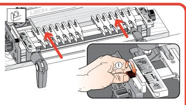
**1-14** Slide the finger assembly onto the support brackets, in the PTD Pin mode and set on the <sup>1</sup>/<sub>2</sub>"[12,7mm] setting. First, tighten both thumbscrews ①.
