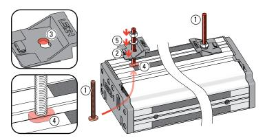
**1-1 Install Side Stops** Insert two clamp T-bolts through the rear jig body holes ① and place a "stepped" rear side stop over each bolt ②, using the rear part of the double-hole ③. Make sure the **bolt's "T" is between the extrusion ribs** ④. Don't forget the steel washer ⑤ and use a ½"[13mm] wrench to tighten the nuts.
