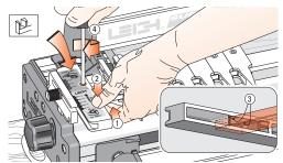
**the scale lock-screw** (4). Repeat at the other end. To maintain correct finger assembly alignment, follow this procedure whenever you remove the scales from the finger assembly.
