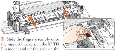
1/2"[12,7mm] setting. First, tighten both thumbscrews ①. Do not lower the assembly onto the finger support board.
