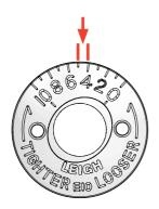
**3-7** One increment of the eBush changes the joint glue line by 0.002"[0,05mm]. Half an increment changes the fit by an incredible 0.001" [0,025mm]. A proper fit will be established with one or two test cuts.
