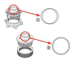
**3-5 Joint Fit Adjustment** The Leigh eBush barrel (A) is elliptical, unlike plain circular template guide bushings (B). When the e10 is rotated, the effective diameter of the barrel changes, allowing fit adjustments as small as 0.001"[0,025mm]. The e10 eBush is included with the jig.
