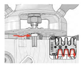
**3-4 How a Guide Bushing Works** The barrel of the guide bushing steers the router and the bits in and around the openings of the template.
