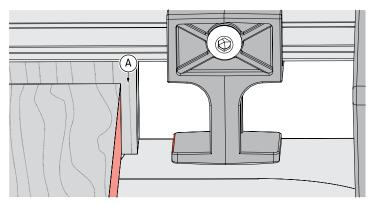
**8-20** Position a backer board <sup>1</sup>/<sub>2</sub>" [13mm] from the board edge (a). This prevents the backer board from interfering with the side stop when the frame is repositioned in the second step. The backer board stays in place for the complete procedure. *Note: Clamps removed for clarity.*
