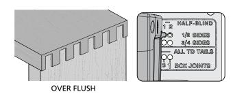
**10-44** Flushness IMPORTANT NOTE: Do not adjust flushness until correct joint tightness in previous steps is achieved. For over flush tails, move the frame pin to a minus ("−") tail position and rout a new test joint. You must re-center the tail board and reposition the side stop every time a reset for flushness is made. Each pin position changes the joint flushness by 0.013"[0.33mm] Record the pin setting for future use. Note: Tail board thickness will not affect flushness.
