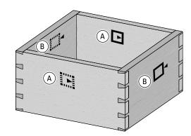
**7-5 Making a Box** Note the symbols indicating the inside or outside of the pin and tail boards. When assembled with the finished pieces properly oriented, any one of the pin ends will fit any one of the tail ends. *Mark the inside faces of the tail boards* (A) **and outside faces of the pin boards** (B).
