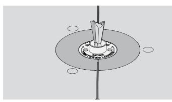
**7-8** With the router unplugged, install the Leigh 80-500 dovetail bit. A Make sure the bit spins freely within the bushing before reconnecting the power.
