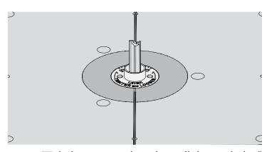
**10-28** With the router unplugged, install the supplied  $\frac{3}{8}$ " Leigh 143-500 bit. For cleaner routing use the optional  $\frac{3}{8}$ " Leigh 173-500 (HSS) or 173-500C (solid carbide) spiral upcut bit, available at leightools.com.  $\triangle$  Make sure the bit spins freely before connecting the power.
