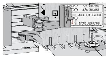
**12-21** Remove pin board 2. Unlatch and move the frame pin to the **No.3 hole, BOX JOINTS** mode and latch the frame. Clamp a socket board against the side stop and rout into all template openings.
