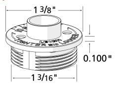
**6-1** The Leigh eBush system is designed around the decades-old Porter Cable/Black & Decker industry standard. Therefore you will likely need to adapt your router table or router table insert plate to accept a Leigh eBush with an insert ring that has a 1<sup>3</sup>/<sub>8</sub>" diameter counter bore. See page 6 for details. Check with your router table or insert plate manufacturer as to what adaptation is required.
