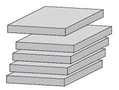
**5-1** Accurate and perfectly aligned joints require stock that is straight, flat, even thickness and equal widths, with square ends and edges. *Note: Plywood is generally unsuitable for routing because of tearout problems.*
