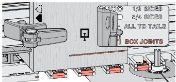
**11-19** Now that your joint tightness has been determined, re-clamp socket board 1 in the jig, move the frame pin to the *No.1 BOX JOINTS* hole and latch frame.
