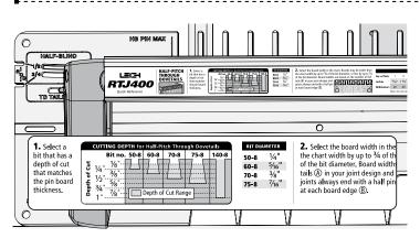
**8-4** Use the Quick Reference strip to determine the correct dovetail bit and guide bushing combination for the board thickness, in this case, the Leigh e10 guide bushing and the optional <sup>3</sup>/<sub>8</sub>" Leigh 70-8 dovetail bit for tails and the optional e7 guide bushing and Leigh 140-8 straight bit for pins.
