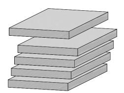
**7-6** Use five similar boards (one for testing) about  $\frac{3}{4}$ " ×  $6\frac{1}{4}$ " by about 12" long [19mm × 159mm × 305mm]. Boards of different thicknesses may also be joined.
