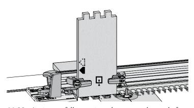
**11-22** Again, carefully rout into the same sockets as before, i.e. 1, 3, 5, 7. Unclamp and flip the board, keeping the same edge against the side stop. Clamp the board and repeat the steps in reverse order. Remove socket board 1 and repeat steps 11-19 through 11-22 for socket board 2. Remove socket board 2.
