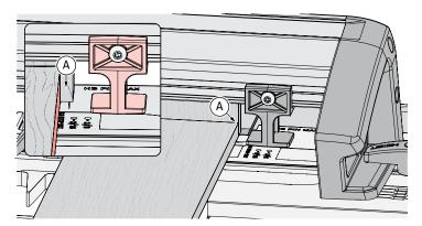
**13-12** Position a backer board at least  $\frac{3}{16}$ " [4.5mm] from the board edge (**A**). This prevents the backer board from interfering with the side stop when the frame is repositioned in subsequent steps. The backer board stays in place for the complete procedure. **Note: Clamp removed for clarity.**
