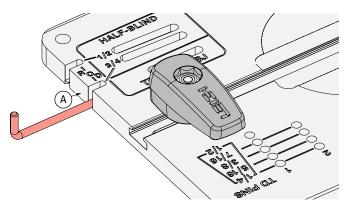
**1-7 Stop Rod:** Insert the stop rod in the <sup>3</sup>/<sub>4</sub>" slot (**A**). The stop rod remains here for all routing operations except half-blind dovetails and box joints. Note: The stop rod may have been shipped in this location.
