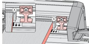
**11-11** Position a backer board <sup>1</sup>/16" [1.5mm] away from the edge of the socket board (**A**). This prevents the backer board from interfering with the side stop when the frame is repositioned in the second step. The backer board stays in place for the complete procedure. **Note: Clamp removed for clarity.**
