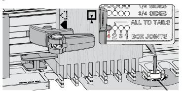
**12-22** Unlatch and move the frame pin to the **No.4 hole, BOX JOINTS** mode and latch the frame. Again, rout into all openings. Unclamp and flip the board, keeping the same edge against the side stop. Clamp it and repeat the routing in reverse order. Remove socket board 1 and repeat steps 12-21 and 12-22 for socket board 2. Remove socket board 2. All four boards are now complete and ready for assembly.
