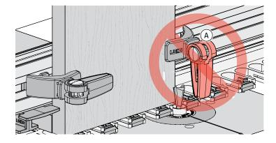
**4-11 Always ensure that the frame clamp levers do not project below the frame when engaged (A)**.
