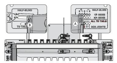
**7-9** Insert the right frame pin in *hole no.2* of the *ALL TD TAILS* mode ⓐ and the left frame pin in the *TD TAILS* & *BJ slot* ⓑ. Securely latch the frame. ⚠ *Always latch the frame to the template after repositioning it.*
