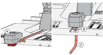
**1-2 Template Latches:** Slide a latch (A) into each end of the template making sure the washer (B) is in the T-slot. Use the hex key (C) through the slot on the bottom of the template to firmly tighten the latches, pulling the hex nuts down into each latch recess. Adjust the latches so they are stiff to slide on the template.
