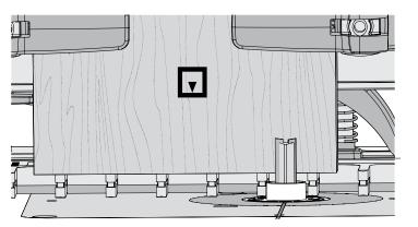
**10-33** Center the tail board over the template so that the side edges are equally spaced over the template fingers and touching flush on the template. Clamp the tail board.
