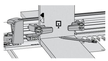
**10-12** Place the end of a socket board on the template and pencil a line on the pin board.
