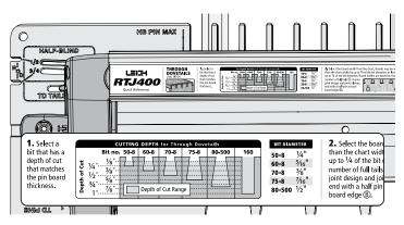
**7-4** Use the Quick Reference strip to determine the correct dovetail bit and guide bushing combination for the board thickness, in this case, the Leigh e10 Guide Bushing and the Leigh 80-500 bit.
