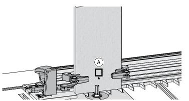
**7-30** Utilizing the final fit setting you determined in Step 7-26 (not the calculated setting in Step 7-27), the two pin boards are now ready for routing. Clamp pin board 1 to the frame against the same side stop with the marked outside face out (A) and the bottom end edge flush on the template. Rout the pins.
