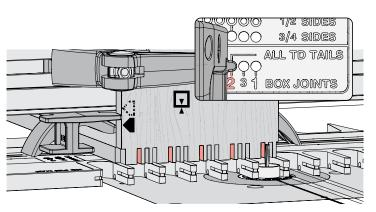
**13-28** Leave the board in place. Unlatch the frame and move the right frame pin to position 2. Rout in every template opening.
