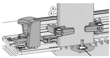
**10-38 Quick Fit Test** To save time and wood, clamp the two 1/2" thick scrap *test* boards in the jig, back to back (A). Rout both boards at the same time. Join the routed boards and make joint fit adjustments in the next three steps. Don't worry about board edge alignment, the test is for joint fit only. **Note:** If you have already done the Quick Fit Test in Step 10-17, use that eBush setting.
