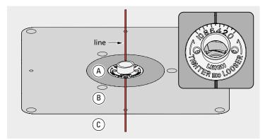
**6-2** Draw a line with a permament pen on the router table, centered on the guide bushing opening at 12 o'clock and 6 o'clock (shown in red for clarity only). This will ensure correct orientation of the eBush to the insert ring (A), the insert plate (B), and the router table (C).
