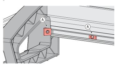
**1-3** Insert the two square nuts into the rear of the frame (A) and slide them to each end of the frame.
