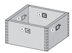
**8-5** Making a Box Note the symbols indicating the inside or outside of the pin and tail boards. When assembled with the finished pieces properly oriented, any one of the pin ends will fit any one of the tail ends. *Mark the inside faces of the tail boards* (A) and outside face of the pin boards (B).
