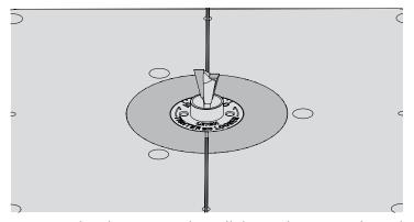
**9-8** Unplug the router and install the Leigh 120-500 dovetail bit. A Make sure the bit spins freely before reconnecting the power.
