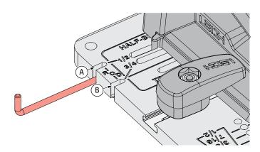
**9-12 The Stop Rod.** For tail boards (sides) from 3/8" [9mm] to 5/8" [16mm] thick, insert the stop rod in the 1/2" slot (A). Note: For tail boards 11/16" [17.5mm] thick or greater, the stop rod is stored in the 3/4" slot (B).
