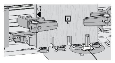
**11-24** Now rout into the second and every alternating even numbered openings, i.e. 2, 4, 6, etc. **Do not remove the board, backer board or the blockers**.
