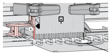
**13-24** Leave the board in place. Move the side stop, with the blocker attached, against the board and tighten it (A).
