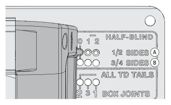
**9-10** NOTE: Tail Boards (drawer side) must be between  $\frac{3}{8}$ " [9mm] and  $\frac{7}{8}$ " [22mm]. For tail boards between  $\frac{3}{8}$ " [9mm] and  $\frac{5}{8}$ " [16mm] thick, use the  $\frac{1}{2}$ " row of holes (**A**). For tail boards between  $\frac{11}{16}$ " [17.5mm] and  $\frac{7}{8}$ " [22mm] thick, use the  $\frac{3}{4}$ " row of holes (**B**).
