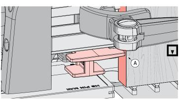
**10-34** Slide the side stop so it lightly touches against the tail board and tighten it. (A).
