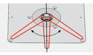
7-27 Re-tighten the eBush nut after each guide bushing adjustment. Rout the other end of the test pin board. Once the fit is correct, add the two eBush settings together and divide by two. **Example:** 5 for tails, 3 for pins.  $(5 + 3 = 8 \div 2 = 4)$ . Record setting "4" on an eBush diagram in the next step. Do not use this new setting for routing this test box, use **only** for future projects.
