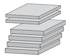
**10-6** Prepare four similar boards  $\frac{3}{4}$ " × 5 $\frac{1}{16}$ " by about 12" long [19mm × 129mm × 305mm]. For the quick fit test you will need two test boards about  $\frac{1}{2}$ " thick. Boards of different thicknesses may also be joined.
