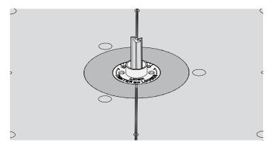
**10-8** With the router unplugged, install the supplied  $\frac{3}{8}$ " Leigh 143-500 bit. For cleaner routing use the optional  $\frac{3}{8}$ " Leigh 173-500 (HSS) or 173-500C (solid carbide) spiral upcut bit, available at leightools.com.  $\triangle$  Make sure the bit spins freely before connecting the power.
