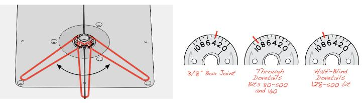
**6-7** Adjust the eBush with the pin wrench. Markings on the eBush indicate which way to turn it for a looser or tighter fit. **Remember, every time you adjust the eBush you must re-tighten the eBush nut.**
