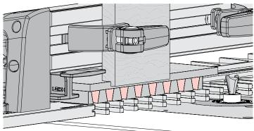
**9-37** Rout in each template opening.  $\triangle$  The eBush must touch one side of the opening as you enter and the other side as you exit.
