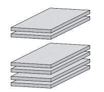
**13-6** Prepare four similar boards <sup>1</sup>/<sub>4</sub>"× 4 <sup>5</sup>/<sub>8</sub>" by about 8" long [10mm × 115mm × 200mm]. For the quick fit test you will need two test boards about <sup>1</sup>/<sub>4</sub>" or <sup>3</sup>/<sub>16</sub>" thick. Boards of different thicknesses may also be joined. *IMPORTANT: Read this whole chapter before routing any boards.*
