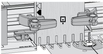
**12-19** Rout into every opening. A The eBush must touch one side of the opening as you enter and the other side as you exit. Do not remove the routed board or the backer board.
