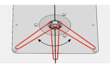
**10-16** Each increment on the eBush changes the joint glue line fit by 0.002" [0.05mm]. Half an increment, a mere 1000th inch! *Re-tighten the eBush nut after each guide bushing adjustment.*
