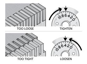
**12-15** Joint Fit Adjustment Keep the same side board edges together. If the joint is too loose, turn the eBush to a higher number, as shown in the next step. If too tight, turn the eBush to a lower number.
