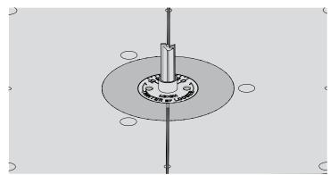
**8-17** With the router unplugged, install the 5/16'' [8mm] 140-8 straight or equivalent spiral bit. A Make sure the bit spins freely within the eBush before reconnecting the power.
