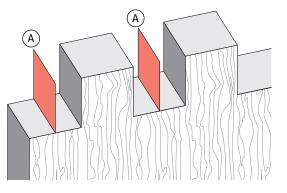
**11-26** Theoretically, there will be nothing left in the sockets, where the bit has passed by twice. However, routing tolerances can leave a very thin "wall" (. This can be quickly removed with a chisel, file, or knife.
