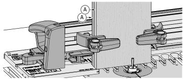
**13-15** Quick Fit Test To save time and wood, clamp the two approx.  $\frac{3}{16}$ " thick scrap **test** boards in the jig, back to back (A). A **Review the remaining steps in this Chapter.** Rout both boards in all four frame pin positions 1, 3, 2 and 4. Join the routed boards and make the joint fit adjustments in the next three steps. Don't worry about board edge alignment, the test is for joint fit only.
