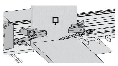
**7-22** Place the edge of the tail board on the template and pencil a line on the pin board.
