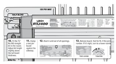
**7-17** As instructed in the Quick Reference strip, always use the ½" [12.7mm] Leigh 160 straight bit or equivalent spiral bit to rout the full pitch through dovetail pins.
