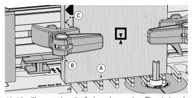
**10-10** Clamp pin board 1 flush on the template (A) with the side edge against the side stop (B). *Always keep the same side edge of the board to the side stop when routing box joints* (C). If the board width is only slightly narrower than the chart width, center the board over the template, clamp in place and move the side stop against the board.
