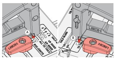
**1-8** The frame is located on the template by a pin on the frame handles. Place the frame on the template by inserting the right frame pin in the *ALL TD TAILS* hole (A) and the left frame pin in the *TD TAILS* & *BJ* slot (B).  $\triangle$  To prevent damage to the frame pin always remove the right frame pin first when lifting the frame handle.
