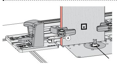
**9-16** Slide the side stop so it lightly touches the tail board and tighten it **(A)**.
