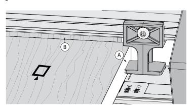
**10-35** Position the pin board against the side stop (A) with the end edge touching *flush against the rear of the tail board* (B), and clamp. *Note: Clamp removed for clarity.*
