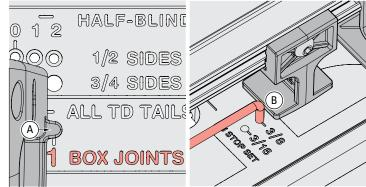
**11-9** Insert the right frame pin in the **No.1 BOX JOINTS** hole (A) and the left frame pin in the matching slot, then latch the frame. Put the short end of the stop rod into the **3/8**" **BJ STOP SET** hole. Slide the side stop to lightly touch the rod (B) and tighten the stop. Store the stop rod in the  $\frac{3}{4}$ " slot.
