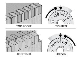
**10-15** Joint Fit Adjustment Keep the same side board edges together. If the joint is too loose, turn the eBush to a higher number, as shown in the next step. If too tight, turn the eBush to a lower number.
