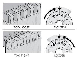
**8-26 Test for Fit** If the joint is too loose, turn the eBush to a higher number with the pin wrench as shown in the next step. If the joint is too tight, turn the eBush to a lower number. Each increment on the eBush changes the joint glue line fit by 0.002" [0.05mm]. Half an increment, a mere 1000th inch!
