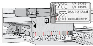
**13-29 Leave the board in place**. Unlatch the frame and move the right frame pin to position 4. Rout in every template opening. Unclamp and flip the board, keeping the same side edge against the side stop. Clamp it and repeat the steps in reverse order. Remove socket board 1. Repeat the procedure for socket board 2. Remove socket board 2. All boards are now complete and ready for assembly.
