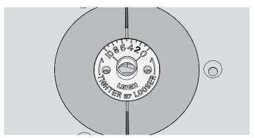
**8-16** Fit the e7 eBush to the router table/router table insert, set to 5.
