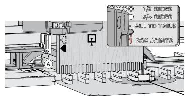
**13-23** Leave pin board 2 in place and do not unlatch the frame. Loosen the side stop and move it away from the board. *Note: The right frame pin should already be in position 1.* Attach one of the blockers to the side stop. Make sure the blocker is seated firmly against the side stop (A).
