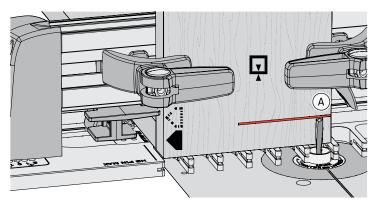
**12-13** Adjust the bit until the tip is level with the center of the pencil line on board 1 ⓐ. *IMPORTANT: Bit height determines the flushness of the joint, so set your bit properly the first time.* Adjustments for flushness if required are at the end of the chapter. ⚠ Double check that the bit still rotates freely.
