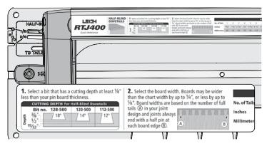
**9-4** Use the Quick Reference strip to determine the correct dovetail bit and guide bushing combination for the board thickness, in this case, the Leigh e10 Guide Bushing and the optional  $\frac{1}{2}$ " 18° dovetail bit.
