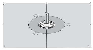
**11-8** With the router unplugged, install the supplied  $\frac{3}{8}$ " Leigh 143-500 bit. For cleaner routing use the optional  $\frac{3}{8}$ " Leigh 173-500 (HSS) or 173-500C (solid carbide) spiral upcut bit, available at leightools.com. A Make sure the bit spins freely before connecting the power.
