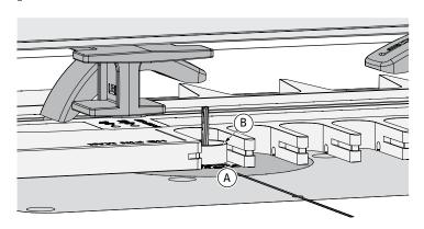
**13-10** Raise the bit above the template and move the template, putting the eBush in the first template opening (a) with the inner edge of the opening (b) touching the bushing.
