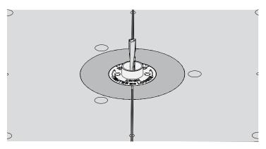
**13-8** With the power disconnected from the router, install the optional  $\frac{3}{32}$ " Leigh 163 bit.  $\triangle$  Make sure the bit spins freely within the bushing before reconnecting the power.
