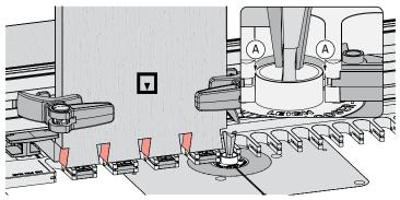
**7-15** Rout in the first and every other opening, 1, 3, 5 and 7. The eBush when set at 5 is slightly narrower than the opening A. A The eBush must touch one side of the opening as you enter and the other side as you exit. Do not twist the jig on the table. Keep the edge of the template square to the center line on the table.
