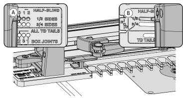
9-9 Insert the right frame pin in the No.0 hole of HALF-BLIND
