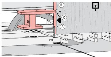
**13-11** Set pin board 1 on the template, touching the  $\frac{3}{32}$ " bit (A). Clamp in place. Move the side stop to touch the board edge (B) and tighten it. The  $\frac{3}{32}$ " box joint requires moving the template from right to left in four steps. Always keep the same side edge of the board to the side stop when routing box joints (C).
