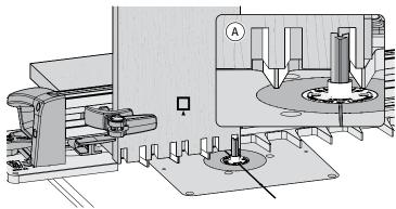
**8-23** A Very carefully, without losing guide bushing contact with the angled finger surfaces (A), rout in and out, both sides of the angled fingers. This a two step process – DO NOT remove the pin board or backer board.
