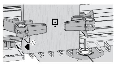
**12-10** Clamp pin board 1 vertically with the side edge against the side stop, the end edge flush on the template. *Always keep the same side edge of the board to the side stop when routing box joints* (A).
