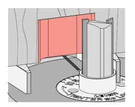
**7-24** Always rout a light climb cut between the template fingers to leave a nice clean shoulder. A climb cut may pull the jig to the right so be sure to control the jig firmly at all times.
