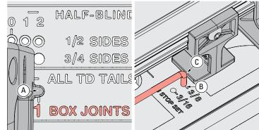
10-9 Insert the right frame pin in the No.1 BOX JOINTS hole (A) and the left frame pin in the TD TAILS & BJ slot. Latch the frame. Put the short end of the stop rod into the 3/8" BJ STOP SET hole (B). Slide the side stop to lightly touch the rod (C) and tighten the side stop. Store the stop rod in the <sup>3</sup>/<sub>4</sub>" slot.
