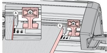
**10-11** Position a backer board  $\frac{1}{16}$ " [1.5mm] away from the edge of the pin board (A). This prevents the backer board from interfering with the side stop when the frame is repositioned in the second step. The backer board stays in place for the complete procedure. *Note: Clamp removed for clarity.*
