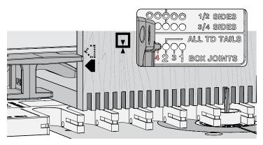
**13-22** Leave the board in place. Unlatch the frame and move the right frame pin to position 4. Rout in every template opening. Unclamp and flip the board, keeping the same edge against the side stop. Clamp the board. Repeat the steps in reverse order. Remove pin board 1. Repeat procedure for pin board 2.
