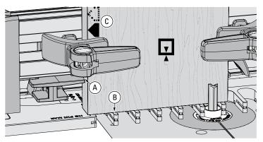
**11-10** Clamp socket board 1 flush on the template **(B)** with the side edge against the side stop **(A)**. *Always keep the same side* **edge of the board to the side stop when routing box joints (C)**. If board width is only slightly narrower than the chart width, center the board over the template, clamp in place and move side stop to touch the board.
