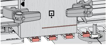
**11-14** This procedure requires routing into alternating template openings. To prevent routing the wrong sockets, insert the supplied blockers into each even numbered opening across the board width, plus one extra.
