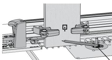
**10-36** The depth of cut (how much the tail board intersects the pin board) is arbitrarily set. Our suggestion is to set the depth of cut about  $\frac{1}{8}$ " less than the thickness of the pin board or in the case of lipped drawer fronts, slightly lower than the lip. In this case our pin board is  $\frac{3}{4}$ ", so mark a line up from the end of the tail board  $\frac{5}{8}$ ".
