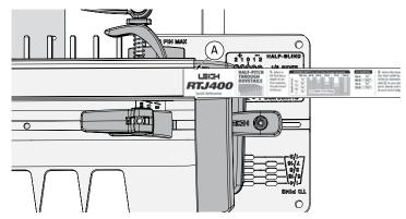
**1-10** If not already in channel, slide the Quick Reference strips into the channel in the top of the jig (A).
