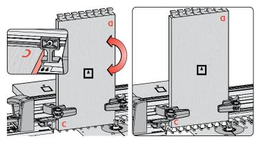
**9-27** Left: Rotate tail board 2 (corner C). Remove pin board 1 and insert pin board 2 (Inset: corner C). Right: Rout in all openings. *Tail board 2 is complete and pin board 2 is half complete*.
