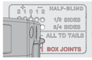
**13-9** Insert the right frame pin in the **No.1 hole**, **BOX JOINTS** mode and the left frame pin in the **TD TAILS & BJ slot** and latch the frame.
