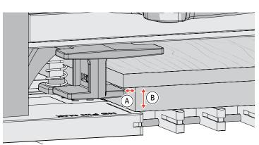
**9-33 Rabbeted Drawer Fronts:** Provided the rabbet on the drawer front is less than <sup>3</sup>/<sub>8</sub>" [9.5mm] wide (A) and more than <sup>3</sup>/<sub>8</sub>" deep (B), the side stop, as previously set on the drawer side, is correctly positioned for the rabbeted pin board.
