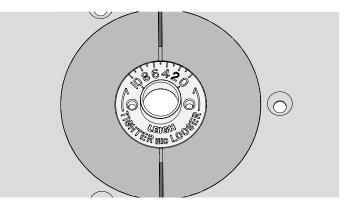
**10-7** Fit the e10 eBush to the router table insert ring, set to 5.
