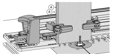
**12-14** Quick Fit Test To save time and wood, clamp the two <sup>1</sup>/<sub>4</sub>" thick scrap *test* boards in the jig, back to back (A). A Review *the remaining steps in this chapter.* Rout both boards at the same time. Repeat again with the frame in the *No.2 hole, BOX JOINTS* mode. Join the routed boards and make joint fit adjustments in the next steps. Don't worry about board edge alignment, the test is for joint fit only.
