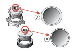
**6-4** The Leigh eBush barrel is elliptical (A), unlike plain circular template guide bushings (B). When rotated, the effective diameter of the barrel changes, allowing fit adjustments as small as 0.001"[0.025mm]. The e10 eBush is included with the RTJ400.
