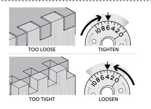
**11-16 Test for Fit** Keep the same side board edges together. If the joint is too loose, turn the eBush to a higher number, as shown in the next step. If too tight, turn the eBush to a lower number.
