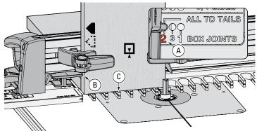
**10-19** Unlatch and move the right frame pin to the *No.2 hole* in the *BOX JOINTS* mode (A). Latch the frame. Clamp socket board 1 against the side stop (B), flush on the template (C).
