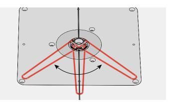
**9-21** Each increment on the eBush changes the joint glue line fit by 0.002" [0.05mm]. Half an increment, a mere 1000th inch! *Re-tighten the eBush nut after each guide bushing adjustment.* **IMPORTANT NOTE:** If the joint is still loose with the eBushing set at 10, measure the depth of cut and make sure it matches Step 9-2.
