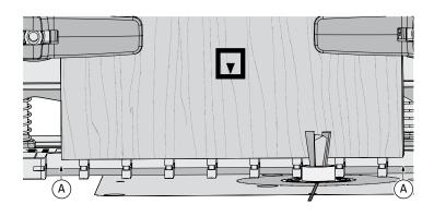
**9-15** Center a **test** tail board over the template so that the side edges (a) are equally spaced over the template fingers and the end edge sits flush on the template. The edge of the board must be positioned halfway into the first opening, otherwise you'll rout into the side stop. Clamp the tail board.
