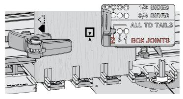
**11-21** Loosen the latches and move the frame pin to the *No.2 BOX JOINTS* hole and latch the frame.
