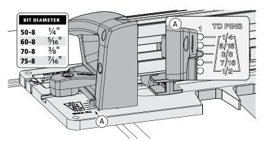
**8-18** Rotate the frame to the *TD PINS* mode. Insert the right frame pin in the *Column 1 hole* that matches the dovetail bit diameter that was used to rout the tails,  $\frac{3}{8}$ " (70-8) in this example (A), and the left frame pin in the matching slot. Latch the frame.
