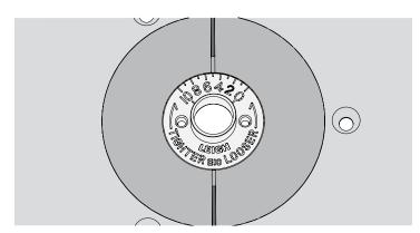
**10-27** Fit the e10 eBush to the router table insert ring. If you have already determined the correct fit in the  $\frac{3}{8}$ " box joint chapter, use that setting, or alternatively use the Quick Fit Test, Step 10-14.
