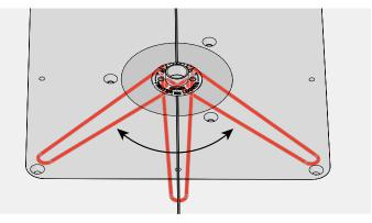
**10-40** Each increment on the eBush changes the joint glue line fit by 0.002" [0.05mm]. Half an increment, a mere 1000th inch! *Re-tighten the eBush after each guide bushing adjustment.*
