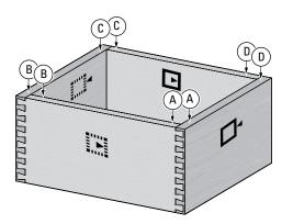
**9-14** When making a box, it is important to label the corners of each board  $(\mathbb{A}, \mathbb{B}, \mathbb{C})$  and  $(\mathbb{D})$ . When routing the corners of the box, both halves of each corner must be in the jig and routed at the same time.
