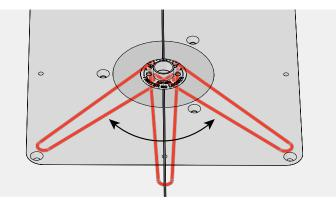
**11-17** Each increment on the eBush changes the joint glue line fit by 0.002" [0.05mm]. Half an increment, a mere 1000th inch! *Re-tighten the eBush nut after each guide bushing adjustment.*
