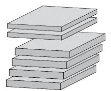
**12-6** Prepare four similar boards <sup>5</sup>/<sub>8</sub>" × 4 <sup>5</sup>/<sub>8</sub>" by about 8" long [19mm × 115mm × 200mm]. For the quick fit test you'll need two test boards about 1/4" thick. Boards of different thicknesses may also be joined. IMPORTANT: Read this whole chapter before routing any boards.
