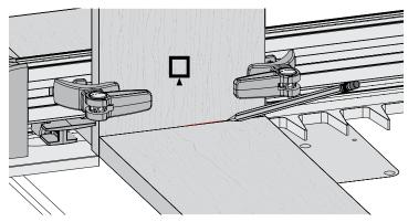
**8-21** Place the end of a tail board on the template and pencil a line on the pin board.
