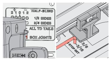
**12-9** Insert the right frame pin in the **No.1 hole, BOX JOINTS** mode and the left frame pin in the **TD TAILS & BJ slot**. Latch the frame. Put the short end of the stop rod into the **3/16" BJ STOP SET** hole. Slide the side stop to lightly touch the rod and tighten the side stop. Store the stop rod in the <sup>3</sup>/<sub>4</sub>" slot.
