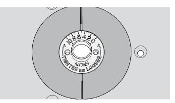
**13-7** Fit the e10 eBush to the router table insert ring, set to 5.
