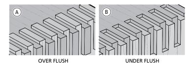
**13-30** If the joint is over flush ⓐ, lower the bit to suit. If the joint is under flush ⓐ, raise the bit to suit. Rout a fresh test joint until fit and flushness are perfect before routing the actual workpieces. ■
