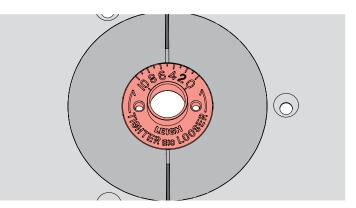
**12-7** Fit the e10 eBush to the router table insert ring set to 5, or if you have already done the quick fit test, use this setting instead.
