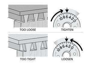
**9-38 Test for Fit** If the joint is *too loose*, turn the eBush to a higher number as shown in the next step, and rout the other end of the test board. If the joint is *too tight*, turn the eBush to a lower number and rout the other end of the test board.
