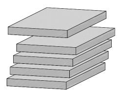
**8-6** Prepare five similar boards (one for testing) about  $\frac{1}{2} \times 6\frac{1}{4}$ " by about 12" long [13mm × 159mm × 305mm]. Boards of different thicknesses may also be joined.
