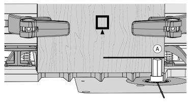
**7-23** Position the jig close to the bit and adjust the bit height until the bit tip is touching the center of the line (a). A Double check that the bit still rotates freely. *IMPORTANT: Bit height determines the flushness of the joint, so set your bit properly the first time.* Adjustments for flushness are near the end of the chapter.
