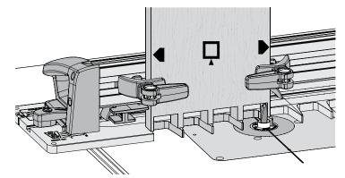
**Note:** Because through dovetail pin and tail boards are 2-2 rotated and clamped with the same face against the frame, both side edges are alternately used against the side stop.
