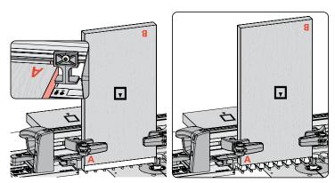
**9-25** Now rout the box. Left: Insert tail board 1 (corner A). Insert pin board 1 (Inset: corner A). Right: Rout in all openings. *Tail board 1 and pin board 1 are half complete.*
