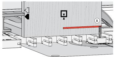
**13-14** Adjust the bit until the tip is level with the center of the pencil line on pin board 1 (a). A Double check that the bit still rotates freely. *IMPORTANT: Bit height determines the flushness of the joint, so set your bit properly the first time.* Adjustments for flushness are at the end of the chapter.
