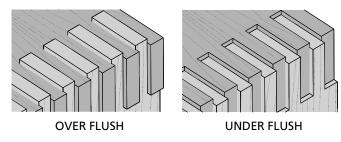
**12-23** Flushness If the joint is **over flush**, lower the bit to suit. If the joint is **under flush**, raise the bit to suit. ■
