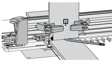
**13-13** Place the end of a socket board on the template and pencil a line on the pin board.
