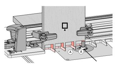
**7-25** Rout out all spaces between the template fingers, being sure the guide bushing touches each side of each finger (A) and all waste is routed between the pins.
