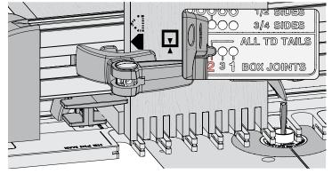
**12-20** Unlatch and move the right frame pin to the **No.2 hole**, **BOX JOINTS** mode, latch the frame. Rout into every opening. Unclamp and flip the board, keeping the same side against the side stop. Clamp it and repeat the steps in reverse order. Remove pin board 1 and repeat steps 12-19 and 12-20 for pin board 2.
