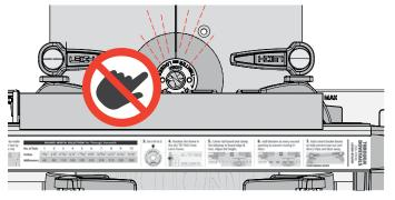
**3-8**  $\triangle$  Using the jig with the handles will ensure your fingers are always safely away from the router bit.
