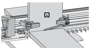
**7-13** Bit height is set using the pin board as a gauge. Place the face of the pin board on the template and pencil a line on the tail board.
