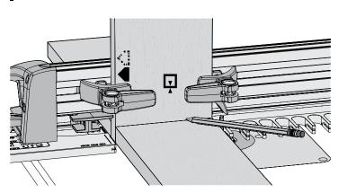
**12-12** Place the end of a socket board on the template and pencil a line on the pin board.
