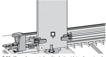
**7-20** Clamp the **test** pin board in the jig with its edge against the side stop (A) with the marked outside face out and the bottom end edge flush on the template. **Note: The side stop was set when routing the tails, so no adjustment is needed**.
