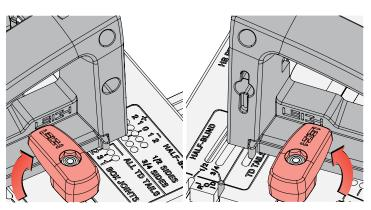
**1-9** Pivot both latches to secure the frame to the template. Double check the latches to ensure they are fully seated. ▲ Only when the frame is latched securely is it safe to lift and or carry the jig by the handles.
