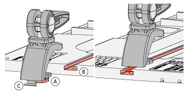
**1-1 Template Clamps:** Insert the clamp T-bolt head (A) into the T-slot at each end of the template (B) followed by the clamp heel (D). Make sure the heels are pointing out at both ends of the template.
