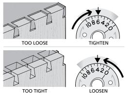
7-26 Test for Fit If the joint is too loose, turn the eBush to a higher number with the pin wrench, as shown in the next step. If too tight, turn the eBush to a lower number. Each increment on the eBush changes the joint glue line fit by 0.002" [0.05mm]. Half an increment, a mere 1000th inch!
