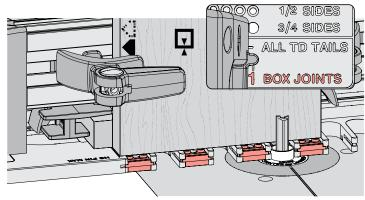
**11-23** Leave the frame latched and the backer board in place. The right frame pin should be in the **No.1 BOX JOINTS** hole. Move the blockers to the odd numbered sockets. Clamp pin board 1 against the side stop.
