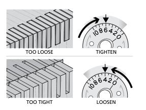
**13-16** Joint Fit Adjustment Join the boards, keeping the same side board edges together. If the joint is too loose, turn the eBush to a higher number, as shown in the next step. If too tight, turn the eBush to a lower number.
