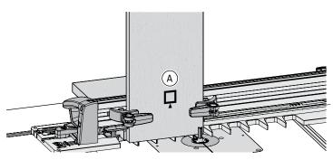
**8-30** Utilizing the final fit setting you determined from Step 8-26 (not the calculated setting in 8-27), the two pin boards are now ready for routing. Reposition the frame to column 1. Clamp pin board 1 to the frame against the side stop with the marked outside face out (A) and the bottom end edge flush on the template. Now rout the first half of the pins. Reposition the frame to column 2 and finish the pins.
