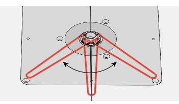
**12-16** Each increment on the eBush changes the joint glue line fit by 0.002" [0.05mm]. Half an increment, a mere 1000th inch! *Re-tighten the eBush nut after each guide bushing adjustment.* If necessary rout further test boards until correct joint fit is achieved, repeating Steps 12-14 through 12-16.
