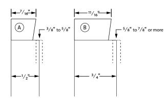
**9-11** When the frame pin and stop rod are in the  $\frac{1}{2}$ " positions, all tails will be this dimension (a), regardless of actual board thickness (dashed line). Similarly, when the frame pin and stop rod are in the  $\frac{3}{4}$ " hole, all tails will be this dimension (b), regardless of actual board thickness.
