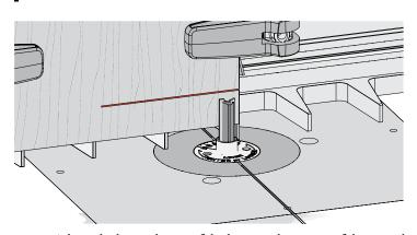
**8-22** Adjust the bit so the tip of the bit is in the center of the pencil line. Double check that the bit still rotates freely. *IMPORTANT:* Bit height determines the flushness of the joint, so set your bit properly the first time. Adjustments for flushness are near the end of the chapter.
