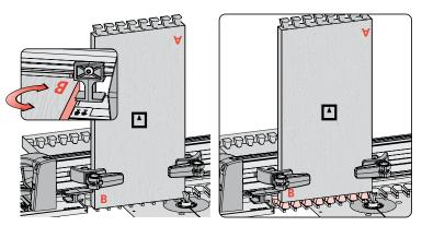
**9-28** Left: Remove tail board 2. Re-insert tail board 1 (corner B). Rotate pin board 2 (Inset: corner B). Right: Rout in all openings. *Tail board 1 and pin board 2 are complete*. All four boards are now complete and ready for assembly. ■
