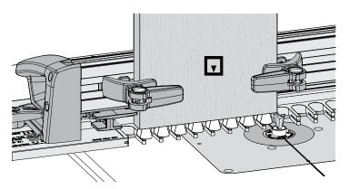
**9-32** Finish the tail board by routing in and out of each template opening, keeping the guide bushing in contact with all template finger surfaces. Remove the tail board.
