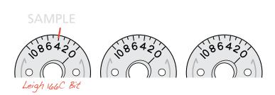
**12-17** On the eBushes above, record the settings you used to achieve perfect joint fit. The first eBush is an example of how to record your setting.
