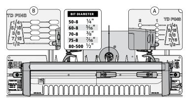
**7-19** Rotate the frame to the *TD PINS* mode. Insert the right frame pin in the *Column 1 hole* that matches the dovetail bit diameter just used to rout the tails, <sup>1</sup>/<sub>2</sub>" in this example (A), and the left frame pin in the matching slot (B). Latch the frame.
