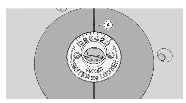
**6-3** All settings for the eBush will be aligned to the line (A) you've drawn on the router table. The line will also help guide the RTJ400.
