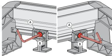
**1-4 Side stops:** Attach the two side stops (A) to the square nuts in the frame using the hex socket button head screws (B), and lightly tighten one side stop at each end of the frame.
