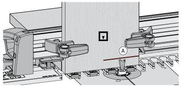
**7-14** Position the jig and tail board close to the bit and adjust the bit height to the center of the line (A). A Double check that the bit still rotates freely. *IMPORTANT: Bit height determines the flushness of the joint, so set your bit properly the first time.* Adjustments for flushness are near the end of the chapter.
