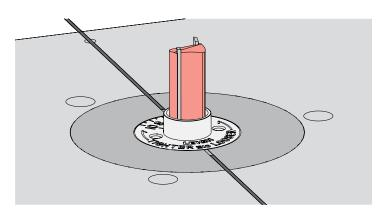
**7-18** With the router unplugged, fit the 160 straight bit to the router and leave the e10 eBush set to 5.  $\triangle$  Be sure the bit spins freely within the guide bushing before reconnecting the power.
