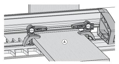
**7-12** Clamp a short scrap backer board (a) horizontally against the tail board to help prevent tear out and direct chips and dust away. This can stay in place for routing of all consecutive tail boards. The scrap board should be at least as thick as the cutting depth of the bit in Step 7-14.
