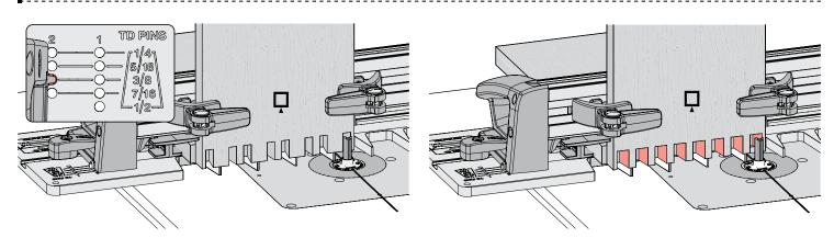
**8-24** Move the frame pin to the **Column 2 hole** of the **3/8" TD PINS** mode. (A) Latch the frame.
