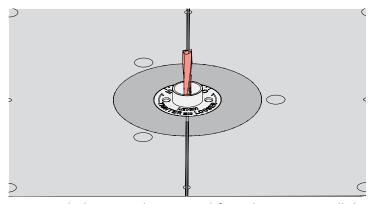
**12-8** With the power disconnected from the router, install the optional <sup>3</sup>/<sub>16</sub>" Leigh 166 (HSS) or 166C (solid carbide) bit. Make sure the bit spins freely in the bushing before reconnecting the power. Optional bits available at leightools.com
