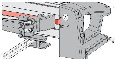
**1-6** When installing the second clamp, insert the T-bolt first and the heel last (A).
