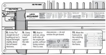
**8-15** Check the Quick Reference strips for the correct guide bushing and bit selection for half pitch pins. *Note:* Half pitch pins always use the optional e7 guide bushing and the optional Leigh 140-8 straight bit. For cleaner routing, use the optional 5/16" Leigh 170 (HSS) or 170C (solid carbide) spiral upcut bit.
