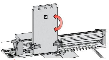
**7-16** A Be sure the router bit has stopped moving before unclamping the tail board. Rotate tail board 1 keeping the same face of the board against the jig. Rout the tails. Repeat 7-15 and 7-16 for tail board 2. Remove the tail board and backer board. Disconnect the power and remove the 80-500 dovetail bit.
