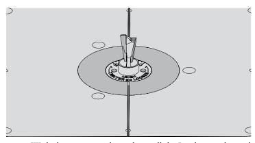
**8-8** With the router unplugged, install the Leigh 70-8 dovetail bit. A Make sure the bit spins freely within the guide bushing before reconnecting the power.
