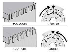
**10-39** Test for Fit If the joint is too loose, turn the eBush to a higher number with the pin wrench as shown in the next step, and *rout two fresh boards.* If the joint is too tight, turn the eBush to a lower number and *rout two fresh boards*.
