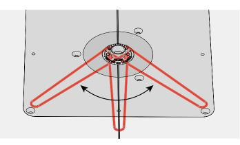
**13-17** Each increment on the eBush changes the joint glue line fit by 0.002" [0.05mm]. Half an increment, a mere 1000th inch! *Re-tighten the eBush nut after each guide bushing adjustment.*
