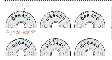
7-28 On the eBushes above, record the settings you used to achieve perfect joint fit. The first eBush is an example of how to record your setting.
