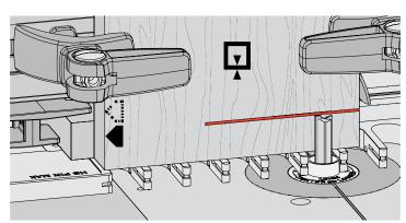
**11-13** Adjust the bit to the center of the line.  $\triangle$  Double check that the bit still rotates freely. *IMPORTANT: Bit height determines the flushness of the joint, so set your bit properly the first time.* Adjustments for flushness are at the end of the chapter.
