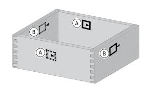
**10-26** Note the symbols indicating the inside or outside of the pin and tail boards. To make a box you will need to mark these symbols on the inside faces of the tail boards (A) and outside faces of the pin boards (B).
