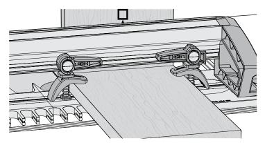
**7-21** Clamp the other end of the scrap backer board horizontally against the back of the pin board.
