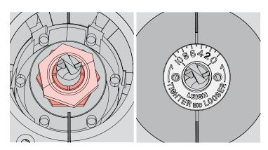
**3-4** Always disconnect the power source and be sure the router has stopped turning before fitting bits, guide bushings or making adjustments. Before reconnecting the router to the power source, make sure the bit and collet revolve freely with and without the guide bushing in place.
