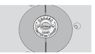
**7-7** Fit the e10 eBush to the router table insert ring. Set the eBush to 5.
