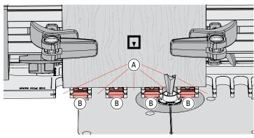
**7-11** You will be routing into the first and every alternate template opening (A). To prevent routing in the wrong opening, fit a supplied blocker (B) into the second and every alternate opening.
