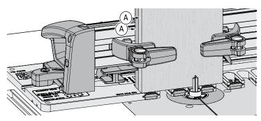
**11-15** Quick Fit Test To save time and wood, clamp the two 1/2" thick **test** boards in the jig, back to back (A). **A Review the** remaining steps in this chapter. Rout both boards at the same time and repeat again with frame in **No.2 BOX JOINTS** hole. Join the routed boards and make joint fit adjustments in the next three steps. Don't worry about board edge alignment, the test is for joint fit only.
