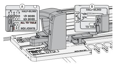
**8-9** Insert the right frame pin in the **No.2 hole** of **ALL TD TAILS** mode (a) and the left frame pin in the corresponding **TD TAILS & BJ slot** (B). Securely latch the frame.
