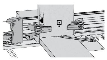
**11-12** Place the end of a pin board on the template and pencil a line on the tail board.
