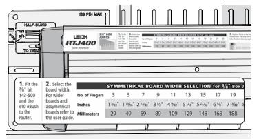
**10-25** Half-blind box joints are made using the same bit and eBush as <sup>3</sup>/<sub>8</sub>" box joints, however the **HALF-BLIND** section of the template is used.
