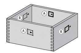
**9-5 Making a Box** Note the symbols indicating the inside or outside of the pin and tail boards. When assembled with the finished pieces properly oriented, any one of the pin ends will fit any one of the tail ends. *Mark the inside faces of the tail boards* (A) **and outside face of the pin boards** (B).
