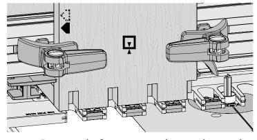
**11-20** Rout into the first opening and every other template opening i.e. 1, 3, 5 and 7. A The eBush must touch one side of the opening as you enter and the other side as you exit. Do not remove the board or the backer board.
