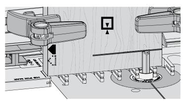
**10-13** Adjust the bit to the center of the pencil line. A Double check that the bit still rotates freely. *IMPORTANT: Bit height determines the flushness of the joint, so set your bit properly the first time.* Adjustments for flushness are at the end of the chapter.
