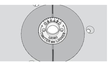
**8-7** Fit the e10 eBush to the router table insert ring, set to 5.
