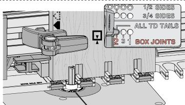
**11-25** Move the frame pin to the **No.2 BOX JOINTS** hole and latch the frame. Rout into the same, even numbered sockets i.e. 2, 4, 6, etc. Unclamp and flip the board. Clamp the board and repeat the steps in reverse order. Repeat steps 11-23 through 11-25 with the second pin board. Remove socket board 2. All four boards are now complete and ready for assembly.
