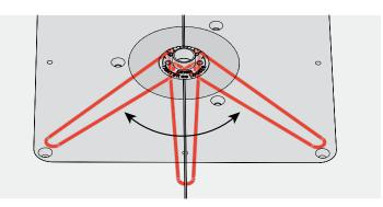
**8-27** Re-tighten the eBush nut after each guide bushing adjustment. Rout a new pin board. Once the fit is correct, add the two eBush settings together and divide by two. **Example:** 5 for tails, 3 for pins  $(5 + 3 = 8 \div 2 = 4)$ . Record setting "4" on an eBush diagram in the next step. Do not use this new setting for routing this test box, **only** for future projects.
