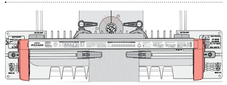
**3-7** Always control the jig with the handles (featured in red) for best routing results, and for safety as shown in next step.
