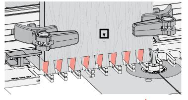
**8-14** Rout the tails in every template opening. A The eBush must touch one side of the opening as you enter and the other side as you exit. Rotate tail board 1 and rout the other end. Repeat routing for tail board 2. Remove the tail board and backer board. *Disconnect the power and remove the e10 eBush & dovetail bit.*
