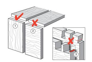
**5-3 (A) Dovetail joints are intended for joining end-grain (D) (D)**
