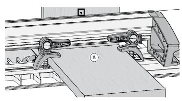
**8-11** Clamp a short scrap backer board (A) horizontally against the tail board to help prevent tear out and direct chips and dust away. This can stay in place for routing of all consecutive tail boards. The scrap board should be at least as thick as the cutting depth of the bit in Step 8-13.
