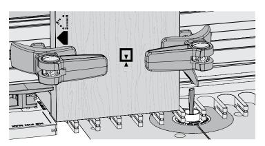
**12-18** Now that your joint tightness has been determined, re-clamp pin board 1 with the side edge against the side stop, the end edge flush on the template.
