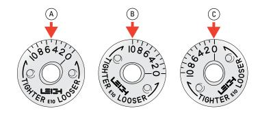
**6-5** All routing starts with the eBush in the No.5 position (a). Turning the eBush toward the No.10 position (b) results in a tighter fit because the guide bushing is now wider. Turning the eBush toward the No.0 position (c) results in a looser fit.
