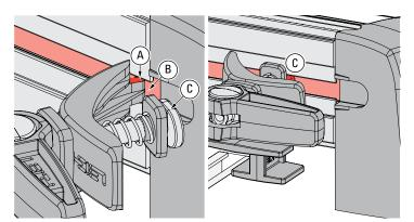
**1-5** Frame Clamps: Insert the heel (A) of a pre-assembled clamp assembly into the end of the frame T-slot (B) followed by the clamp T-bolt (C), and slide the clamp to the other end of the frame. Note: The clamp arm spring washers are under tension. They may need to be pulled away from the T-bolt to aid in ease of assembly.
