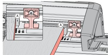
**12-11** Position a backer board at least  $\frac{3}{6}$ " [4.5mm] from the board edge (A). This prevents the backer board from interfering with the side stop when the frame is repositioned in the following steps. The backer board stays in place for the complete procedure. *Note: Clamp removed for clarity.*
