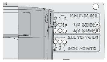
**10-30 NOTE:** Use the ½" row **(A)** for tail boards 3%" [11mm] to %" [16mm] thick, and the 3¼" row **(B)** for tail boards 1½6" [17.5mm] to 7%" [22mm] thick.
