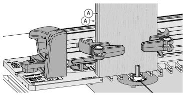
**10-38 Quick Fit Test** To save time and wood, clamp the two ½" thick scrap **test** boards in the jig, back to back (a). Rout both boards at the same time. Join the routed boards and make joint fit adjustments in the next three steps. Don't worry about board edge alignment, the test is for joint fit only. **Note:** If you have already done the Quick Fit Test in Step 10-17, use that eBush setting.
