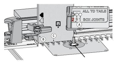
**10-19** Unlatch and move the right frame pin to the **No.2 hole** in the **BOX JOINTS** mode (A). Latch the frame. Clamp socket board 1 against the side stop (B), flush on the template (C).
