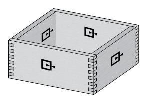
**10-5 Making a Box** Note the symbols indicating either side of the pin and socket boards can face in or out. With box joints, the same edge of the board goes against the side stop.
