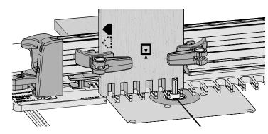
**10-18** Now that your joint tightness has been determined, re-clamp pin board 1 in position and rout into all of the openings.
