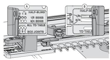
**10-29** Insert the right frame pin in the  $\frac{1}{2}$ " HALF-BLIND "0" pin hole (A) and the left frame pin in the  $\frac{1}{2}$ " HALF-BLIND slot (B). Latch the frame. Note: The HALF-BLIND pin hole settings refer only to the thickness of the pin board (drawer side).
