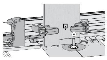
**10-37** Adjust the bit to the center of the line **(A)**.
