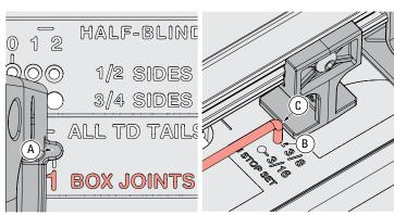
**10-9** Insert the right frame pin in the **No.1 BOX JOINTS** hole (a) and the left frame pin in the **TD TAILS & BJ** slot. Latch the frame. Put the short end of the stop rod into the **3/8" BJ STOP SET** hole (a). Slide the side stop to lightly touch the rod (a) and tighten the side stop. Store the stop rod in the 3/4" slot.
