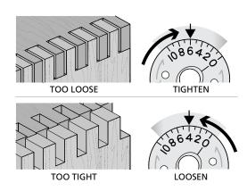
**10-15 Joint Fit Adjustment** Keep the same side board edges together. If the joint is too loose, turn the eBush to a higher number, as shown in the next step. If too tight, turn the eBush to a lower number.
