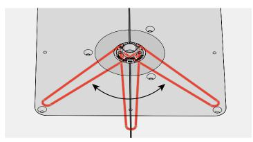
**10-40** Each increment on the eBush changes the joint glue line fit by 0.002" [0.05mm]. Half an increment, a mere 1000th inch! **Re-tighten the eBush after each guide bushing adjustment.**
