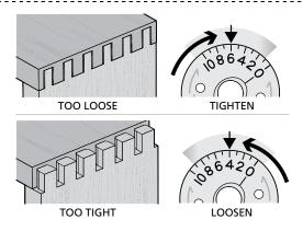
**10-39 Test for Fit** If the joint is too loose, turn the eBush to a higher number with the pin wrench as shown in the next step, and *rout two fresh boards*. If the joint is too tight, turn the eBush to a lower number and *rout two fresh boards*.
