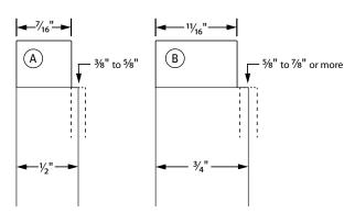
**10-31** When the frame pin and stop rod are in the  $\frac{1}{2}$ " positions, all tails will be  $\frac{7}{16}$ ", dimension (a), regardless of actual board thickness (dashed line). Similarly, when the frame pin and stop rod are in the  $\frac{3}{4}$ " hole, all tails will be  $\frac{11}{16}$ ", dimension (b), regardless of actual board thickness.
