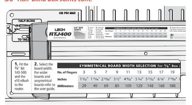
**10-25** Half-blind box joints are made using the same bit and eBush as 3/8" box joints, however the **HALF-BLIND** section of the template is used.
