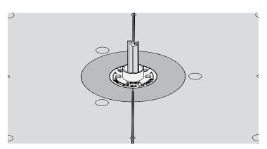
**10-8** With the router unplugged, install the supplied <sup>3</sup>/<sub>8</sub>" Leigh 143-500 bit. For cleaner routing use the optional <sup>3</sup>/<sub>8</sub>" Leigh 173-500 (HSS) or 173-500C (solid carbide) spiral upcut bit, available at leightools.com. ⚠ Make sure the bit spins freely before connecting the power.
