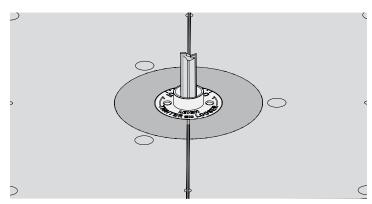
**10-28** With the router unplugged, install the supplied ¾" Leigh 143-500 bit. For cleaner routing use the optional ¾" Leigh 173-500 (HSS) or 173-500C (solid carbide) spiral upcut bit, available at leightools.com. ⚠ Make sure the bit spins freely before connecting the power.
