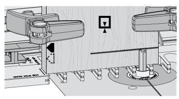
**10-13** Adjust the bit to the center of the pencil line. ⚠ Double check that the bit still rotates freely. *IMPORTANT: Bit height determines the flushness of the joint, so set your bit properly the first time.* Adjustments for flushness are at the end of the chapter.
