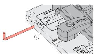
**10-32** The Stop Rod. For tail boards from  $\frac{3}{8}$ " [11mm] to  $\frac{5}{8}$ " [16mm] thick, insert the stop rod in the  $\frac{1}{2}$ " slot A. Note: For tail boards 11/16" [17.5mm] thick or greater, the stop rod is stored in the  $\frac{3}{4}$ " slot B.
