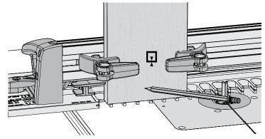
**10-36** The depth of cut (how much the tail board intersects the pin board) is arbitrarily set. Our suggestion is to set the depth of cut about ½" less than the thickness of the pin board or in the case of lipped drawer fronts, slightly lower than the lip. In this case our pin board is ¾", so mark a line up from the end of the tail board ½".
