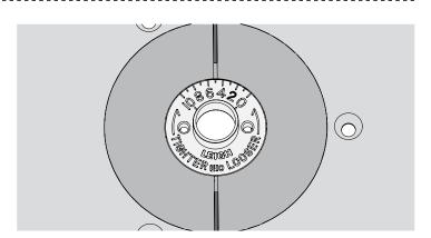
**10-7** Fit the e10 eBush to the router table insert ring, set to 5.
