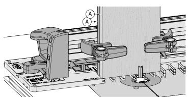
**10-14 Quick Fit Test** To save time and wood, clamp two ½" thick scrap boards in the jig, back to back (A). First review the remaining steps up to 10-20. Rout both boards at the same time. Test the boards for joint fit, and make joint fit adjustments (steps 10-15 to 10-17). Don't worry about board edge alignment, the test is for joint fit only.
