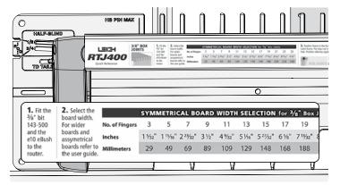
**10-4** Use the Quick Reference strip to determine the correct straight bit and eBush combination.
