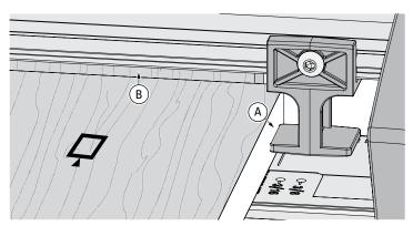
**10-35** Position the pin board against the side stop A with the end edge touching *flush against the rear of the tail board* B, and clamp. *Note: Clamp removed for clarity.*
