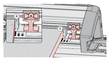
**10-11** Position a backer board ½16" [1.5mm] away from the edge of the pin board (a). This prevents the backer board from interfering with the side stop when the frame is repositioned in the second step. The backer board stays in place for the complete procedure. **Note: Clamp removed for clarity.**
