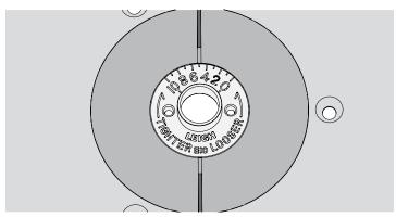
**10-27** Fit the e10 eBush to the router table insert ring. If you have already determined the correct fit in the <sup>3</sup>/<sub>8</sub>" box joint chapter, use that setting, or alternatively use the Quick Fit Test, Step 10-14.
