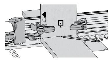
**10-12** Place the end of a socket board on the template and pencil a line on the pin board.
