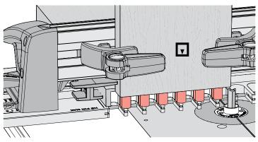
**10-43** Finish routing in and out of all template openings. ⚠ The eBush must touch one side of the opening as you enter and the other side as you exit.
