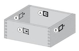
**10-26** Note the symbols indicating the inside or outside of the pin and tail boards. To make a box you will need to mark these symbols on the inside faces of the tail boards (A) and outside faces of the pin boards (B).
