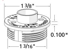
**6-1** The Leigh eBush system is designed around the decades-old Porter Cable/Black & Decker industry standard. Therefore you will likely need to adapt your router table or router table insert plate to accept a Leigh eBush with an insert ring that has a 13/8" diameter counter bore. See page 6 for details. Check with your router table or insert plate manufacturer as to what adaptation is required.
