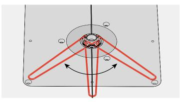
**6-7** Adjust the eBush with the pin wrench. Markings on the eBush indicate which way to turn it for a looser or tighter fit. Remember, every time you adjust the eBush you must re-tighten the eBush nut.
