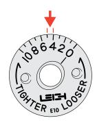
**6-6** One division of the eBush changes the joint glue line by 0.002" [0.05mm]. A perfect fit will be established with one or two test cuts.
