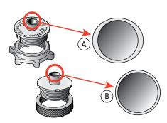
**6-4** The Leigh eBush barrel is elliptical (a), unlike plain circular template guide bushings (b). When rotated, the effective diameter of the barrel changes, allowing fit adjustments as small as 0.001"[0.025mm]. The e10 eBush is included with the RTJ400.
