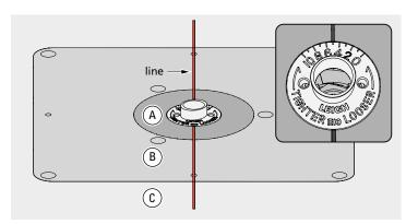
**6-2** Draw a line with a permament pen on the router table, centered on the guide bushing opening at 12 o'clock and 6 o'clock (shown in red for clarity only). This will ensure correct orientation of the eBush to the insert ring (A), the insert plate (B), and the router table (C).
