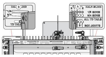
**4-3** The template must be used perpendicular to the line drawn on the table. In this orientation, pin holes (A) and corresponding slots (B) are for half-blind dovetails, through tails and box joints.
