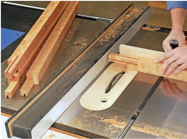
Cut the legs' offset tenons at the table saw with a wide dado blade, backing the workpieces up against a long auxiliary fence attached to the miter gauge. Mark these cuts clearly to avoid confusion and possible mistakes.
