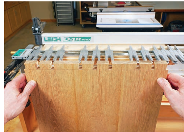
The best way to truly evaluate what a dovetail pattern will look like is to cut a full-size sample on a scrap piece. It enables you to see the interplay of positive and negative spaces as well as the joint's pin and tail balance.
