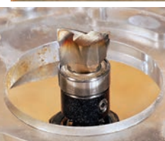
A shop-made, clamp-on routing jig makes hinge leaf mortises quick and accurate to mill with a short piloted mortising/pattern bit (inset). The jig also guides a chisel for squaring up the corners of these mortises.
