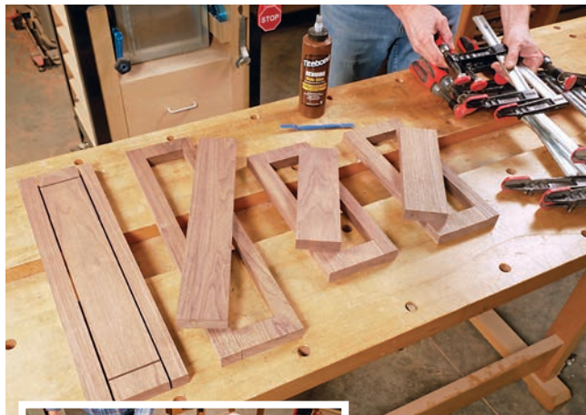
The author cut the rails and stiles for each inner frame from single boards, with the stile grain running width-wise. It enabled stronger edge-grain glue joints and continuous grain pattern as well as simpler final surfacing of the frames (inset).
