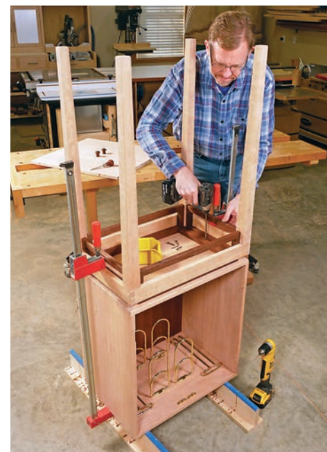
Install the Rev-A-Shelf hardware and fasten the leg base to the cabinet to set these screw locations. Then remove the hardware and leg base for final finishing.
