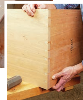
Flipping the guide finger assembly over to its "closed" side and switching to a straight bit in the router resets the jig for milling pins and tail sockets. Fine-tuning at this step can produce a piston fit of the parts (inset).
