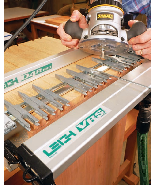
Through dovetail joints machined on Leigh's D4R Pro Dovetail Jig begin with the tail cuts, made on the "open" side of the jig's adjustable guide fingers with a dovetail bit. Here, the author mills one of his final workpieces.
