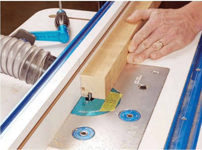
Plow 1/4"-wide, 5 1/4"-long grooves into two adjacent faces of the legs at the router table. Mark the cutting limits of the bit clearly on the table's surface so you'll know where to begin and end these cuts.
