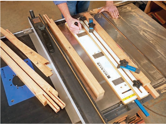
Two inside faces of each leg are tapered, reducing the legs to 1 1/4" at the bottom. Be very clear about which faces receive these cuts. A moment's lapse in attention can lead to a scrapped part and a complete do-over.
