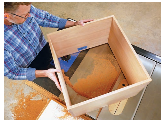
Rather than teetering a handheld router on the back edges of the cabinet carcass to mill rabbets for the back panel, the author carried this operation out on a large, table saw-mounted router table instead.
