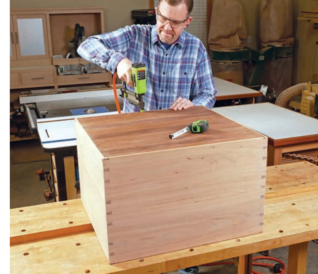
After squaring up the rounded corners of the back rabbets, cut and install a plywood back panel on the cabinet with 1 1/4", 18-gauge brad nails.
