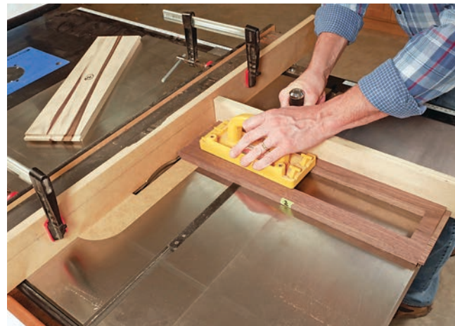
Raise 1/4"-thick, 3/8"-long tongues on the ends of the inner frames with a wide dado blade at the table saw or on the router table. Also pictured here is one of the four full-size test pieces for the inner frames.
