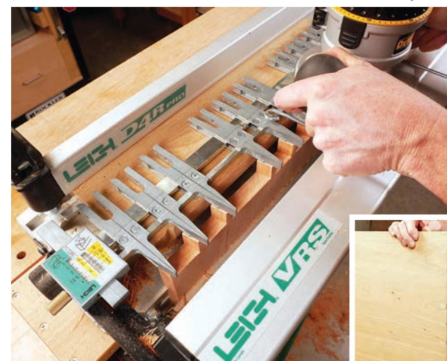
Flipping the guide finger assembly over to its "closed" side and switching to a straight bit in the router resets the jig for milling pins and tail sockets. Fine-tuning at this step can produce a piston fit of the parts (inset).
