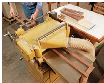
The author cut the rails and stiles for each inner frame from single boards, with the stile grain running width-wise. It enabled stronger edge-grain glue joints and continuous grain pattern as well as simpler final surfacing of the frames (inset).
