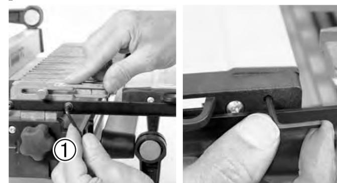
**15.** Now firmly tighten the other two button head screws ①. The hex key stows in the right hand end of the VRS.
