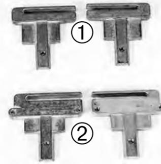
**11. D1600 Owners:** First, remove the existing cast support brackets ①. You will be using the new type ② that came with your VRS16.
