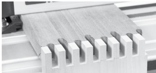
**19.** For maximum efficiency, always back-up vertically mounted workpieces with a backer board. This not only prevents chips and dust exiting the rear of the board, it also aids in preventing tear out from the rear of the workpiece.
