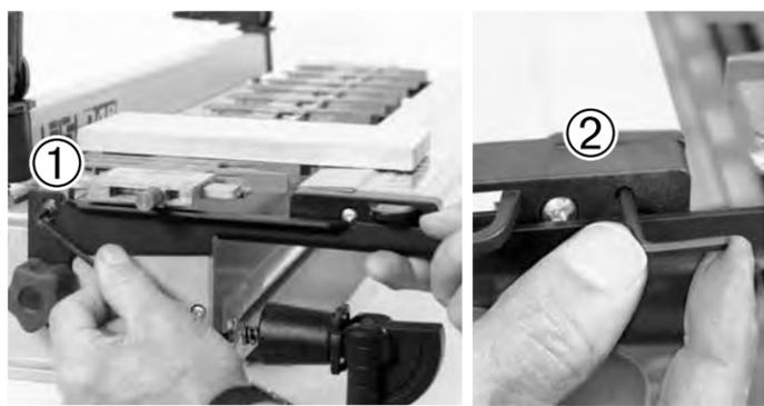
**10.** Now firmly tighten the two button head screws ①. The hex key stows in the right hand end of the VRS ②. **After installation, when raising and lowering the combined VRS & finger assembly, always take the weight at the inner end of the brackets ③, not at the VRS ends.** *Note: The VRS height may need to be reset when using Isoloc or Finger Joint Templates.*
