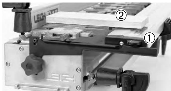
**8.** With the jig finger assembly mounted and lowered onto its support board; install the VRS onto the steel brackets ①. Lay a piece of flat board on the finger assembly and extending out over the top of the VRS extrusion ②.
