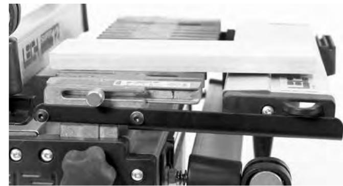
**13.** Mount the finger assembly and lower it onto its support board. Install the VRS onto the steel brackets and lay a flat board on the finger assembly, extending out over the top of the VRS extrusion.
