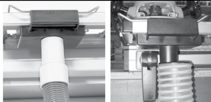
**18.** Attach the shop vacuum hose direct to the collector nozzle or use one of the two hose adaptors supplied. Keeping the front clamps vertical and turning the large hose adaptor away from the clamp allows full router travel.
