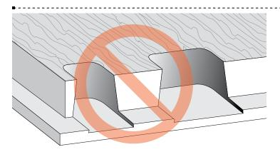
11-7 Make sure you select a dovetail bit that has a working depth of cut less than the rabbet height. Otherwise, you will rout into the rabbet.
