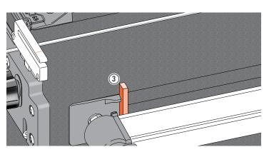
**11-5** Stick the block ① to the jig face with double-sided tape, making sure it touches the side stop.
