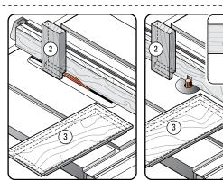
**11-2 Rabbeted Pins** You will need to block the scrap stop in the front of the jig out from the jig's front face by exactly the width of the rabbet ①.
