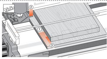
**11-4** If the rabbet width ① is greater than the top side stop width of 3/8" ②, the drawer side (tailboard) must be blocked away from the front side stop (see 11-5) by exactly the width of the rabbet minus 3/8" ③. For example, a 5/8" rabbet ① would require the tailboard to be offset by an additional 1/4" ③.
