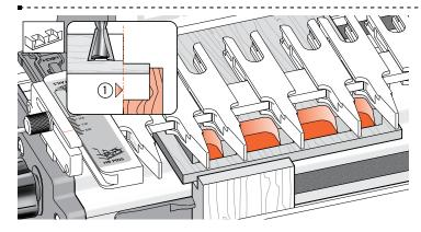
**11-3** This brings the pin ends exactly in line with the front jig face ①, ensuring that the scale reading is accurate.
