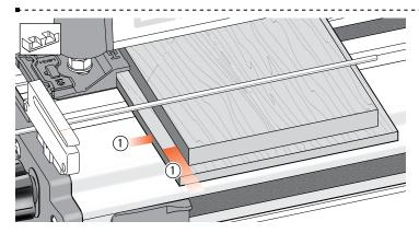
**11-1** Provided the drawer front lip is  $\frac{3}{8}$ " [9,5mm] or less in each direction ①, you can mount and rout rabbeted drawer fronts **and sides** exactly the same way as flush drawer fronts, except...
