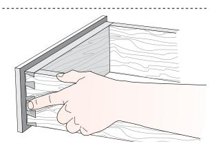
11-8 It is difficult to clean up the drawer sides and front corner after assembling a rabbeted drawer, so make sure the fit is flush before you complete the drawers See 9-28 to 9-30. ■
