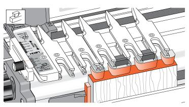
**11-6** The drawer side will now be stepped in from the side stop by the width of the rabbet, bringing the sockets in line with the pins.
