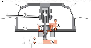
**7-3** When fitting a bit to the router ①, fit the shank as far into the collet ② as possible. Always rout with the collet as close to the guidebush as possible. Usually you can't securely grip the collet nut with a wrench ③ if the collet is at its optimum low position. Fit the bit so that the remaining travel ④ between collet and guidebush ⑤ will let the bit reach the required depth of cut ⑥.
