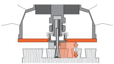
**7-6** Depth of cut is **not** the distance the bit projects from the router base. This is **bit projection** ②. This user guide generally refers to depth of cut. Bit projection ② is always .500"[12,7mm] more than depth of cut.
