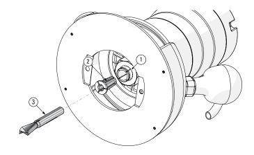
**7-2** Routers used on Super Jigs must have a ½" or 8mm collet ①. All Super Jig bits have 8mm shanks. Routers with ½" collets must use the ½" to 8mm collet reducer ② supplied with the jig. The collet reducer ② is inserted in the router collet ① (chuck) and the 8mm shank bit ③ is inserted in the collet reducer. Routers with 8mm collets do not require a collet reducer.
