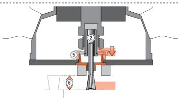
**7-4** Tighten the collet ② securely and lower the collet to adjust the depth of cut ⑥, but make sure the collet does not contact the guidebush ⑤.
