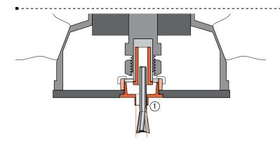
**7-7** Ideally, the router collet (and bit) should be concentric (centered) to the guidebush as in figure 7-5. Regrettably, this is often not the case; the bit can be off center (eccentric to) the guidebush ①. The illustration shows the problem highly exaggerated. The good news: bit to bush alignment doesn't affect joint fit or flushness; both are "adjusted out" in normal jig setup.
