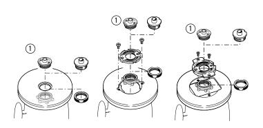
**7-1** Fit the e7-Bush ①. One is included with your Super Jig. Some guidebush adaptors may have to be modified to allow adjustment rotation of the e7-Bush in the base. *See page 67*. If the e-Bush is incompatible with your router, any 7/16"[11,1mm] guidebush (min. depth ½" see page 67) will work for all but box joints on the Superjig.
