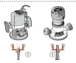
**7-8** Bit to guidebush offset may change when the router motor is unclamped from the base when changing bits or making bit height adjustments. Concentricity problems can also arise if two routers are used for through dovetails, (one for pins; one for tails). Routers with different bit to guidebush offsets ② (misalignment shown highly exaggerated)...
