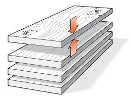
**6-1** It is vital for accurately aligned joints that stock used on the Superjig should be prepared straight, flat, of even thickness and equal widths, with square ends and edges. *Note that plywood is generally unsuitable for routing because of tearout problems.*
