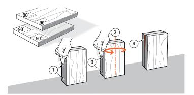
**6-2** Check for squareness: stand both pieces vertically on a flat surface. Make sure side edges are flush at bottom and top ①. Turn one piece around on its end ②. If side edges are flush top to bottom ③, the boards are square. If not, ④; cut two that are.
