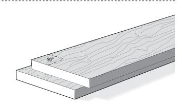
**6-4** You will want to test the jig, so prepare some  $\frac{3}{4}$ " x  $5\frac{1}{2}$ "[20x140mm] boards. Cut them to length as you need them for the jig tests you want to perform. Use them for practice with the jig's various joint modes so you can see how the different modes work. Remember, though, that two boards of different thicknesses can be joined just as easily.
