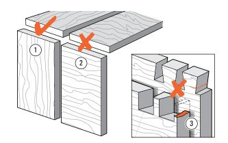
**6-3** Dovetail joints are intended for joining end-grain to end-grain ①. Attempting to rout dovetails in side grain ② will not work because:
