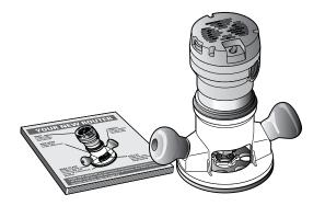
**5-1** Read the user guide that came with your router. It is essential to understand the router manufacturer's instructions completely. Always operate variable speed routers at the fastest possible speed.
