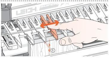
2-2 To practice adjusting the guidefingers, put a board in the front clamp. Always raise the finger assembly slightly, approximately <sup>1</sup>/16"[2mm] above the spacer board and/or workpiece ①. This is essential to allow the guidefingers to move freely on the guidefinger bar and ensures that the fingers will be level and flush when locked up. Move the guidefingers by pushing on the middle to slide them along the guidefinger bar.
