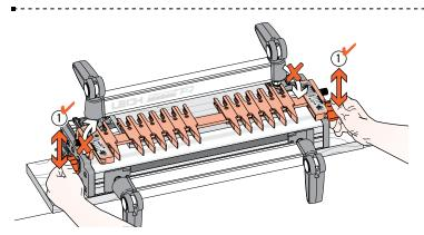
Practice with the finger assembly height adjustment. Loosen 2-1 the support bracket knobs and hold them firmly. Raise and lower the assembly evenly, keeping it level ①, and tighten the knobs to lock it at various heights. Do not raise or lower only one end of the finger assembly.
