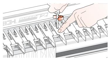
**2-5** Always tighten unused guidefingers before routing, as router vibration may cause loose screws and finger lock parts to fall out and be lost.
