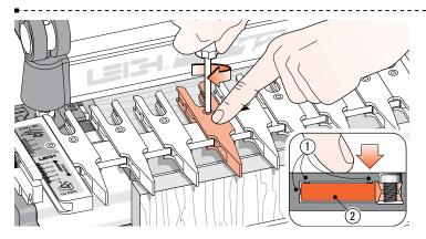
**2-3** Loosen about half the guidefingers and practice unlocking, moving, positioning and re-locking them. Always press on the center of the guidefinger when tightening the screws. This ensures that the small pads 1) on the inside of the finger contact the face of the finger bar 2 and keeps all the fingers level.
