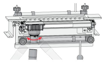
**Step 12** The swivel action vacuum port accepts a 1½" (38mm) diameter hose. Attach your shop vacuum hose to the dust collection port on the vacuum box assembly.
