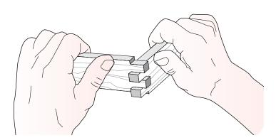
**9-3** Test for fit. Don't worry about board alignment, it's only the fit you're testing. Adjust the **e-Bush** by trial and error and rout more pairs of scrap board ends as required.
