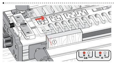
**7-3** Set the template pin on **L**. Clamp a scrap piece vertically in the jig front with its top end slightly above the jig body ①. Clamp a box front horizontally with the inside face  $\square$  away from the jig body, and the front end edge against the scrap board.
