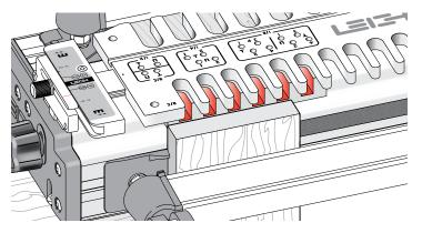
**7-5** Rout a test piece to test the scale setting for joint flushness and adjust the template in or out to produce the required flush fit.
