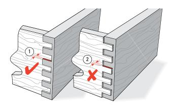
**7-6** The drawer front pins should project through the side sockets by no more than  $\frac{1}{64}$ "[0,25mm] for clean-up ①. If the sides project ②, adjust the template inward to suit.
