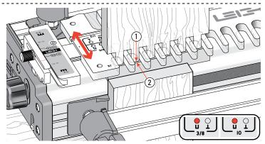
**7-4** Place one of the routed box sides vertically through the template with the rounded part of the fingers in the rounded guide crotches. Adjust the template so the front face of the side board ① is  $\frac{1}{16}$ "[1,5mm] in from the end edge of the box front ②. Lock the scales on the same setting at both ends.
