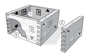
**7-8** Square half-blind box joint boards must be assembled with the inside faces inwards ① but unlike normal box joints, the sides edges may be up or down ②. So you can decide on the preferred board orientation before marking and routing the box bottom grooves ③. You will probably need to clamp in both directions when gluing-up.
