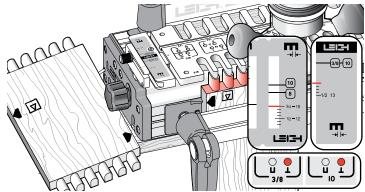
**7-2** Set the template pin on the  $\bot$  setting and the scales to the thickness of the box sides, e.g.  $\frac{3}{4}$  [20mm] shown here. Rout the box side ends vertically in the front clamp.
