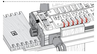
**7-7** When satisfied with the flushness fit, rout all the ends of the box fronts and backs in this mode.
