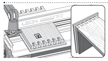
**7-9** Rabbeted Half-Blind Box Joints Rabbeted half-blind workpieces do not require blocking on D4R and SuperJigs if the rabbet is 3%" or less.
