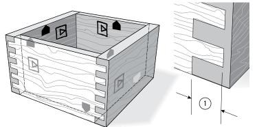
**7-1 Half-Blind Joints** Unlike normal box joints, the inside faces of half-blind box joint boards always face away from the jig body, and alternate edges are placed against the side stop. Set the depth of cut ① to about ½8"[3mm] less than the drawer-front thickness. Use only the "Symmetrical" board widths for half-blind joints.
