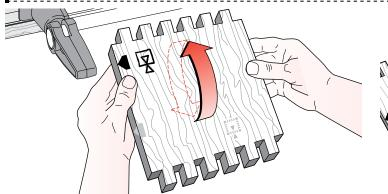
**6-13** All square box joint boards (for boxes or end-on-end joints) are clamped alternately face in and face out **P**, always with the same side edge against the side stop.
