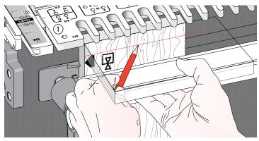
**6-6** Clamp the workpiece against the left-hand side stop; end edge flush under the template. Either face can be out **1**. Mark and adjust depth of cut to suit the board's thickness. Use the board to be joined to mark the depth of cut. Templates have pin holes ① on the left end to allow routing wide boards at the right hand end or a different comb size.
