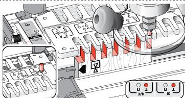
**6-8** Rout one end of a scrap board. Make sure to touch the guidebush on both sides of each template opening.
