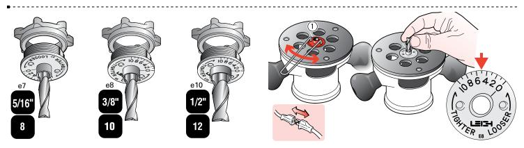
**6-3** Select the correct **e-Bush** and bit combination for the comb size to be used. The bit size is the same as the designated comb size.
