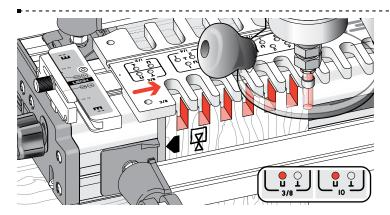
**6-9** Remove the template pin and move the template to position **U**, then refit the pin. Rout the mating board.
