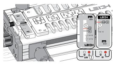
**6-5** Set the scale on the comb size to be used (example here;  $\frac{3}{8}$ "[10mm] comb ①. Position the template with the template pin in position **L** ②. *Remember, position the template pin at the opposite end of the template out of the way of the router.*
