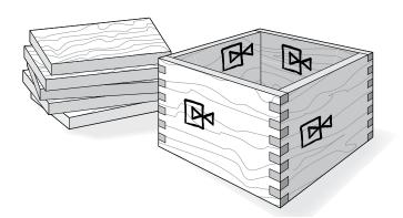
**6-1** Always use scrap boards to test for fit. Scrap width and thickness is not critical. Let's rout some simple box joints. These general instructions apply to any of the comb sizes. Rout single corners to test joint fit. *Note: This chapter combines instruction for joint procedures and joint fit. Follow through step by step the first time, but there is also a "quick fit test" method; see 9-2.*
