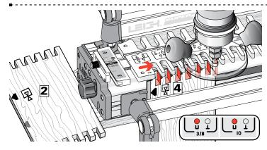
6-15 Rout both ends of boards 2 and 4 in position **L** Keep the same edges to the side stop.
