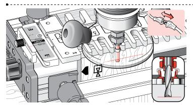
**6-7** Adjust the bit to cut at the centre of the pencil line. Make sure the collet will not rub on the guidebush.
