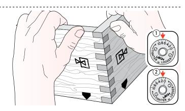
**6-10** Test the two boards for fit. Adjust the **e-Bush** by trial and error and rout more pairs of test boards to achieve the desired fit. Remember, turn the **e-Bush** "up" to a higher number for a tighter joint ① and "down" for a looser joint ②.
