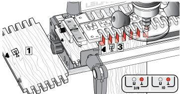
**6-14** Rout both ends of boards **1** and **3** in position **⊥**. Be sure to keep the same edges to the side stop.
