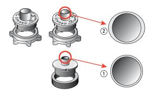
**4-1** Unlike plain circular template guidebushes ①, the e-Bush is elliptical ②. This innovation effectively changes the guidebush "active diameter" when it's rotated, and provides benefits not possible with a plain round guidebush. The F18 and F24 Templates include two Leigh e-Bushes\*: e8 for 3/s"[10mm] combs, and e10 for 1/2"[12mm] combs; the F3 includes those plus the e7 for 1/6"[8mm] comb.
