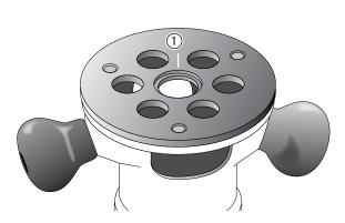
**4-5** Establish the orientation in which you normally hold and operate the router on the jig. Now, up-end the router in the same orientation. Make a small scratch line or permanent ink mark on the router base or e-Bush adaptor at the 12 o'clock position ①.
