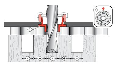
**4-6** With the e-Bush ① turned to "10" in the base ② the active "diameter" is increased, allowing less side-to-side movement, and resulting in smaller sockets and larger pins. A tight fit! Scale and movement are exaggerated in this sequence of illustrations.
