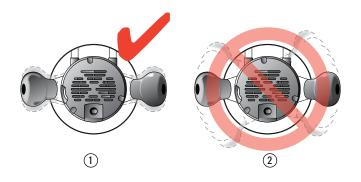
**4-4** Here's how it works. In normal use, the operator does not rotate the router more than a few degrees either way ①. In fact, because of potential bit-to-bush eccentricity problems it is advisable to minimize router rotation on jigs ②.
