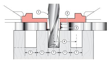
**4-2 Joint Fit and Joint Pitch** Box joints routed with standard sized straight bits ① and standard sized guidebushes ② against straight guide surfaces ③ on pitch centres exactly two times the bit diameter ④ will guarantee a loose fitting joint. Bits, guidebushes and templates are manufactured with necessary plus/minus tolerances and the router will have some degree of run-out, or "wobble".
