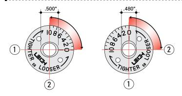
**4-3** The e-Bush (e8 illustrated) fits to the router base or to a guidebush adaptor in the base. *See Appendix I*. The ellipse or oval shape major axis ① is ~.500", and minor axis ② ~.480" [12,7 x 12,2mm]. Turning the e-Bush 90 degrees in the router base changes the active guide size by .020"[,50mm] providing infinite adjustment and recordable settings for perfectly fitting box joints.
