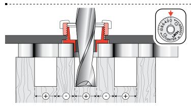
Turning the e-Bush to zero allows more side-to-side router/ bit movement, and more wood removal, producing larger sockets and smaller pins, and thus a loose fit.
