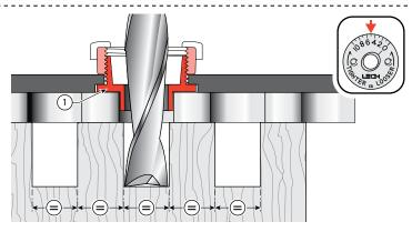
**4-8** A few trial-and-error test cuts and e-Bush adjustments will allow you to establish the correct pin and socket sizes for a perfect fit. Note: One division of the e-Bush changes the joint glueline interface by two thousandths of an inch, that is, 0.002" or 0,050mm.
