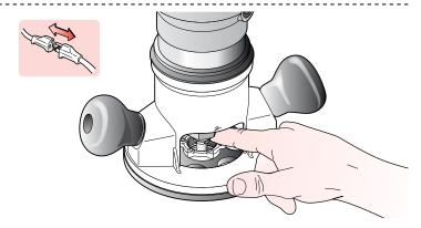
**2-4** Always disconnect the power source from the router when fitting bits or guidebushes, or making adjustments.
