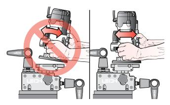
**2-5** Do not tilt the router on the jig. Keep the router flat on the jig assembly. Note: The optional Leigh VRS attachment prevents router tilting.
