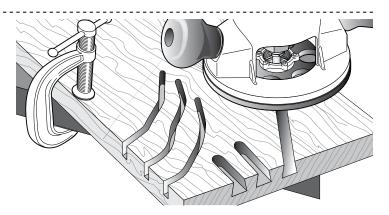
**2-8** If you have never used your router before, be sure to follow the router manufacturer's instructions for its use. Make plenty of simple open-face practice cuts *without a guidebush* before you try to use the router on the Leigh jig. You must, of course, always use a guidebush when routing on the Leigh Jig.
