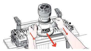
**2-6** If you insist on removing the router from the jig while it is still revolving, always pull it straight off the jig horizontally, and do not raise or lower the router until it is completely clear of the jig.
