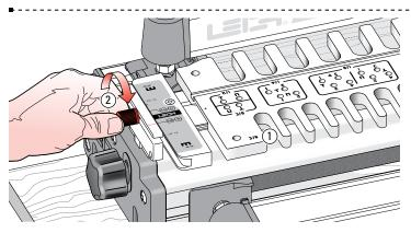
**1-3** Slide the template onto the support brackets, with the  $\frac{3}{8}$ "[10mm] comb toward you ① and set on the  $\frac{3}{8}$ "[10mm] setting.
