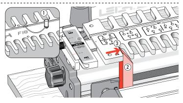
**1-4** Align the template so that its centre hole aligns with the hole in the bar and firmly insert the template pin ①. Angle trim the end of a straight block and clamp it tight against the left stop; the top protruding into the last  $\frac{3}{8}$ "[10mm] opening ②. Move the combined assembly to the right until the left side of the opening touches the block ③. Taking care to not move the template assembly...
