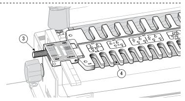
**1-10** Slide the template assembly onto the jig support brackets with the  $\frac{3}{8}$ " &  $\frac{5}{16}$ " [10 & 8 mm] combs toward you and lower it gently onto the jig's spacer board ④. Make sure the scale reading is the same on both scales, e.g.  $\frac{1}{2}$ ", then tighten the thumb screws ③.
