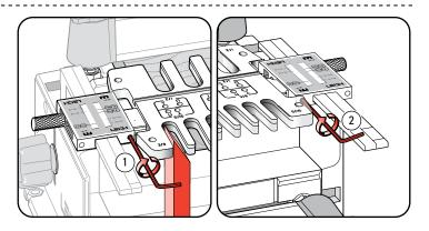
**1-12** ...tighten both scale set screws ① and ②. Remove the block and your Leigh F3 is ready to use. All 4 combs are now registered. **F3M owners:** Note the left set screw will be covered by the template, so tighten the right set screw first. Then remove the block and move the template to tighten the left set screw. ■
