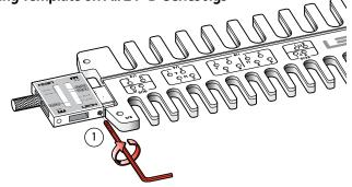
**1-9** Loosen the scale bar set screw ①, at each end of the template.
