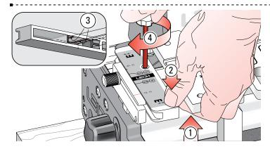
**1-5** ...pull up on the template bar ① while pushing down on the scale ② to ensure the bar is touching the two registration pads ③ inside the scale. Maintain pressure and tighten the scale lock-screw ④. Repeat at the other end. Remove the block and your template is ready to use. **To maintain correct template alignment, follow this procedure whenever you remove the scales from the finger assembly.**
