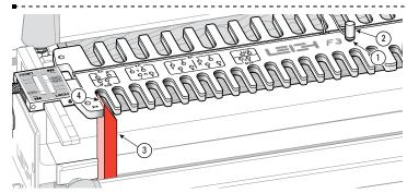
**1-11 Centering the F3** Align the template so its center hole ① aligns with the hole in the bar. Insert the template pin ② with a gentle twist to seat it. Trim the end of a straight block at a 45° angle, then clamp it against the left sidestop and up into the first template opening ③. Move the combined assembly so the left side of the opening touches the block ④. Note: The angled portion of the block should not touch the template. Taking care to not move the template assembly...
