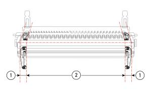
**1-8** Before installing the F3/F3M on any 24" D-series jig with adjustable side stops, set and index the stops according to the jig's user guide. Are the stops  $1^1/2^{"}$ [38mm] in from each end of the jig body extrusion ① and  $24^1/8^{"}$ [613mm] apart ②? If not, do it now.
