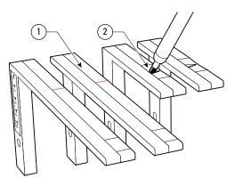
**1-7 D1258, D1258R and D3 jig owners:** If you already own the Leigh Mortise and Tenon Attachment, fit its extended support brackets ① and use for all finger joint and dovetail procedures. If not, mark the arrow pointers on the standard support brackets ② with a dark felt pen. Some D4 and D4R Jig owners already have extended brackets. Late model D4R brackets are shorter.
