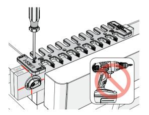
**4-13** Clamp the beam in the vice with the PINS side facing you. With the PINS side of the template toward you, place it on the beam and align it with the pre-drilled holes. Use a screwdriver to attach the template with the included screws. Do not tighten the screws yet! See Step 4-14.
