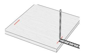
4-18 Depth of Cut Select a board at least 13-1/4" [330mm] wide and 1/2"[12,7mm] to 3/4"[19mm] thick. Length is not important as long as it can be clamped safely in the vice.
