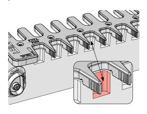
**4-23** Remove the jig from the board.
