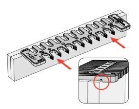
**4-5** With the **PINS** side of the template facing you, lay it flat on the top of the beam and slide it backwards until the positioning ridges contact the edge of the beam. Center the template left to right. The template is now positioned correctly.
