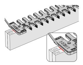
**4-7** Use the left edge of the template as a guide and draw a pencil line completely across the top of the beam.
