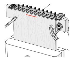
**4-25** Unclamp the board, flip it end for end, keeping the depth of cut lines facing you and reclamp it in the vice.
