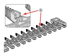
**4-4** The **PINS** side of the template has positioning ridges molded into the underside.
