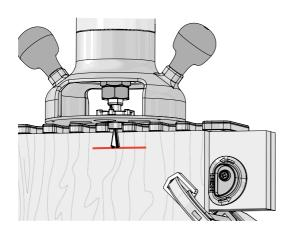
**4-26** Place the router on the jig and adjust the bit until the tip is at the depth of cut line.
