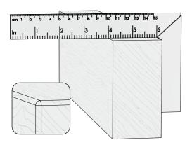
**4-15** As a last resort, you can use a straight, flat 19"[483mm] piece of common 2x4. However this may generate a lot of tearout on the beam. Since a 2x4 has rounded corners, preparation is required. **Note:** the finished thickness must be 1-1/2"[38mm].
