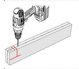
**4-11** Use a drill press or hand drill with a 3/32" bit to drill pilot holes at all screw hole locations on the top of the beam and at the side stop positioning marks.
