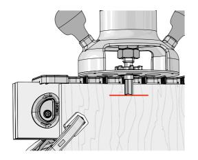
**4-21** Place the router on the jig and adjust the tip of the bit up or down until it's at the center of the line.
