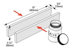
4-2 Making the Beam We recommend laminating two pieces of MDF: 3/4"[19mm] x 3-1/2"[90mm] x 19"[483mm]. Clamp the glued pieces together and set aside to dry. Be sure the top edges are flush and free of glue residue. Alternate materials may be used, eg, a common 2x4 in North America, however the finished thickness must be 1-1/2"[38mm]. See Step 4-14 for special instructions. If you are making dovetails using narrow boards, see Step 5-66.
