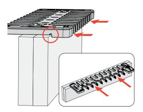
**4-14** Make sure the positioning ridges (see Step 4-5) are held against the beam while tightening the screws.
