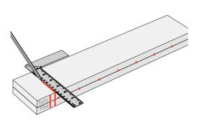
**4-9 Mark layout lines for the side stops.** Place the beam flat on the workbench with the *TAILS* side up. Use a square and draw a line perpendicular from the side stop positioning mark on the top of the beam.
