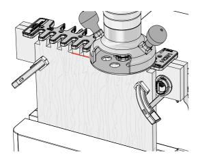
**4-27** Hold the router firmly and rout through the board and into the beam, in each template opening.
