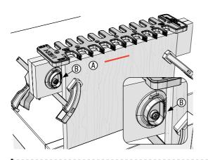
**4-20** With the **PINS** side of the jig facing you, place the jig on the board (a). Slide the jig to the right until the side stop touches the left edge of the board (b) and clamp the jig in place.
