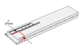
**4-10** Next, draw a horizontal line, 2" [51mm] down from the top of the beam. Make sure the horizontal line intersects the vertical line. This is the mounting point for the side stops.
