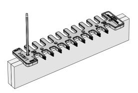
**4-6** Use a pencil and mark the location of all screw holes on the top of the template. Hold the template in place and proceed to the next step.
