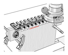
**4-22** Hold the router firmly and rout through the board and into the beam, in each template opening.
