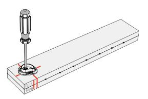
**4-12** Place the beam on the workbench with the *TAILS* side facing up. Align the center of a side stop with the pilot hole and attach it using an included screw. Use a screwdriver, not a power drill, to attach the side stop.
