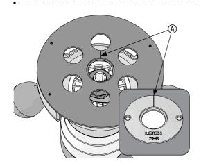
**3-11** Make a small scratch line on the router base or eBush adaptor, at the 12 o'clock position. This will be a reference line for all eBush settings **(A)**.
