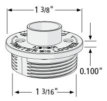
**3-2 The Leigh eBush System** is designed around the 1-3/8" industry standard. Some routers accept the Leigh eBush directly. Many routers require the use of a guide bushing adaptor. If your router requires an adaptor, please see Chapter 7, Guide Bushing Adaptor Selection, or visit leightools.com/guide-bushings-adaptors.
