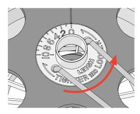
**3-12** Install the *e10-Bush* in the router base and use the pin wrench to align the 0 to the reference line. The 0 setting is only used for beam preparation in Chapter 4, Mounting & Assembly.
