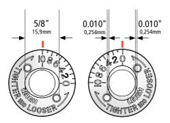
**3-6** The effective diameter of the e10 is 5/8"[15,9mm] at the 10 position. Rotating the eBush to the 0 position reduces the effective diameter by 0.020"[0,5mm].
