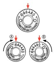
**3-8** Test routing always starts with the eBush set at 5 This allows adjustment for a tighter or looser fit. Turning the eBush toward the 10 position (a) results in a tighter fit. Turning the eBush toward the 0 position (b) results in a looser fit. Be sure to retighten the eBush nut after each adjustment.
