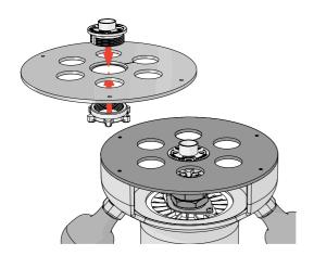
**3-3** Routing on the TD330 requires a router fitted with the included e10 eBush.
