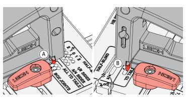
1-8 The frame is located on the template by a pin on the frame handles. Place the frame on the template by inserting the right frame pin in the ALL TD TAILS hole (A) and the left frame pin in the TD TAILS & BJ slot (B). To prevent damage to the frame pin always remove the right frame pin first when lifting the frame handle.
