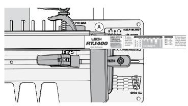
**1-10** If not already in channel, slide the Quick Reference strips into the channel in the top of the jig **(A)**.
