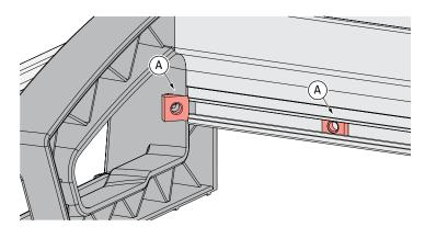
**1-3** Insert the two square nuts into the rear of the frame (A) and slide them to each end of the frame.
