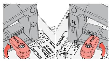
1-9 Pivot both latches to secure the frame to the template. Double check the latches to ensure they are fully seated.
