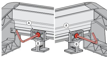
**1-4 Side stops:** Attach the two side stops (a) to the square nuts in the frame using the hex socket button head screws (b), and lightly tighten one side stop at each end of the frame.
