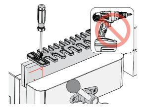
**4-13** Clamp the beam in the vice with its 3/4" side facing you. Position the template on the beam with the 3/4" side of the template facing you. Align it with the pre-drilled holes.
