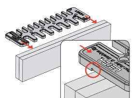
**4-4** With the 3/4" comb facing you, lay the template flat on the beam and center it left to right. Slide the template forward until the ridges on the underside of the 1/2" comb contact the back of the beam. The template is now positioned correctly.
