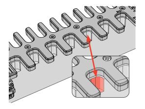
**4-23** There will now be a clean groove in each template opening on both sides of the beam.
