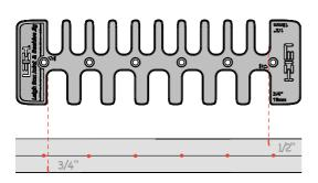
**4-7** Remove the template and mark 3/4" and 1/2" beside the lines, to indicate which is the 3/4" and which is the 1/2" side of the beam.
