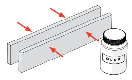
**4-1 Making the Beam** We recommend laminating the two pieces of 3/4" MDF. Place the glued pieces in a vice or use clamps to hold them together. The template will be attached to the top of the beam, so be sure the top edges are flush and free of glue residue. Set aside to dry completely. Alternatively, a common 2x4 may be used. See step 4-15 for special instructions.
