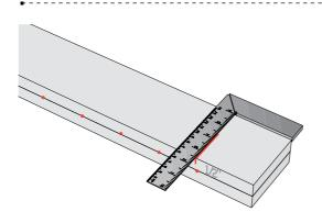
**4-8** Mark layout lines for the side stops. First, place the beam flat on the workbench with the 1/2" side of the beam facing up. Use a square and draw a vertical line down from the positioning mark on the top of the beam.
