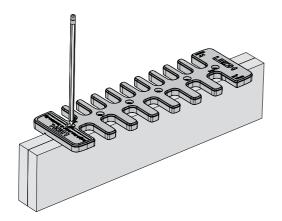
**4-5** Use a pencil and mark the location of all screw holes on the top of the template. Hold the template in place and proceed to the next step.
