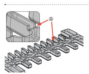
**4-3** The 1/2" comb has positioning ridges (A) molded into the bottom side of the template.
