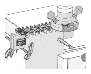
**4-22** Hold the router firmly and rout through the board and into the beam, in each template opening. Be sure the guide bushing touches the left side of each template opening on the way in and the right side on the way out.
