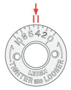
**3-7** One increment of the eBush changes the joint glue line by 0.002"[0.05mm]. Half an increment changes the fit by an incredible 0.001"[0.025mm]. A perfect fit will be established with one or two test cuts.
