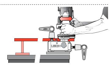
**15-14** When placing long horizontal boards in the rear clamp, make sure the rear end of the board is supported to prevent unnecessary racking of the jig.
