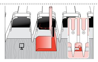
**15-3** Climb rout from left to right from the rear of the cut. Take care to control router.
