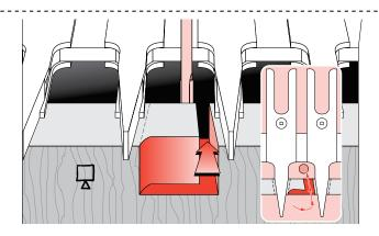
Rout through on the right side until the bit is clear of the workpiece. Move the bit to the left side and climb cut left to right.
