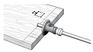
**15-6 Preventing TD Pins Tearout** To help prevent tearout at the back bottom part of a straight cut, scribe a line with your marking gauge across the back of the pin board at exactly the depth of cut.
