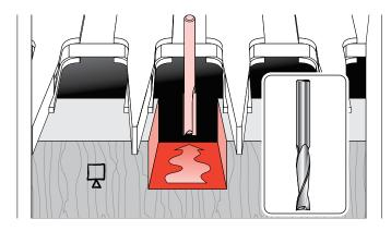
**15-5** Rout away the rest of the waste. Note: Spiral up-cut straight bits (inset) generally rout more smoothly than the two-flute carbide-tipped bits. If you want to try them, you should be aware that while the high-speed steel bits take a better edge, they are much less durable than the more costly solid carbide type (Leigh bits 170 HSS or 170C solid carbide).
