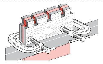
**15-10** For vulnerable or that last piece of exotic wood, clamp horizontal scrap pieces to the front and back of the work piece. Make sure clamps are below the bit depth.
