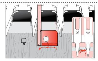
**15-1 Through Dovetail Pins** With the straight bit, carefully climb-rout from right to left. Make sure you control the router firmly when climb routing.
