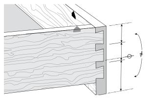
**12-2** An *asymmetrical* joint has a deliberately uneven layout of pins and tails desired for a project design; for example, this dropfront drawer. The half-pin at the bottom of the drawer is much wider than the top half-pin. As the top edges of the front and sides are flush, it makes sense to use these edges against the side stops at each end of the jig. Here's how.
