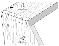
**12-11** Note: If, in the slant-front desk example, the pins were in the desk top and the tails in the sides, then all the parts would be routed in the opposite ends of the jig to those shown in the previous steps.
