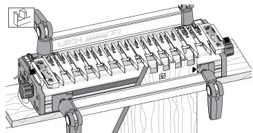
**12-8** To lay out the joint at the right end of the jig, turn the left hand tailboard (like a book page) against the right side stop. Lay out the fingers over the pins you just cut.
