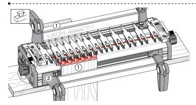
**12-13** However, if this is not an option, the unattractive edge can be hidden from view at the bottom of drawers. Simply rout the right front and left rear drawer corners on the left side of the jig 1, and then...
