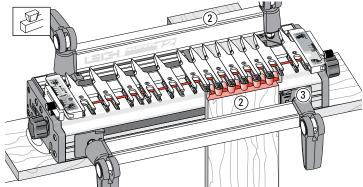
**12-14** ... the left front and right rear drawer corners on the right side of the jig ②. The Spacer is used to offset the drawer sides at both ends of the jig ③. ■
