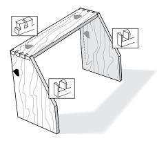
**12-5** Another example of asymmetry is the top corners of a slant-front desk. The joints themselves may be symmetrical, but they must be routed on opposite ends of the jig because the sloped front edges will not register accurately against the fixed vertical side stops.
