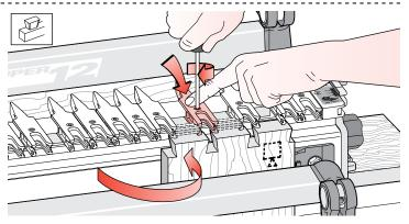
**12-4** Turn one tailboard (like turning a page in a book) to the right end of the jig. Now lay out the fingers at the right end to match the sockets already routed. Now simply rout the left front corner (tails and pins) on the right side of the jig.
