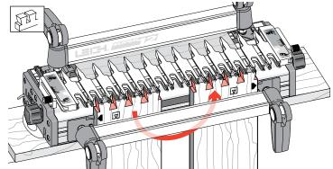
**12-10** Rotate the finger assembly to TD Tails mode. Clamp the tailboard in the left side of the jig and rout the tails. Then rotate the board and clamp against the right side stop to rout the tails in the other end.
