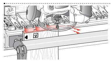
**12-3** Mount the right-hand drawer sides and pins on the left end of the jig for routing, and...
