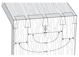
**12-1** By *symmetrical* we mean a joint that looks or is approximately symmetrical about its center line but is probably not, and need not be precisely symmetrical. Using the Leigh jig, it is easy to cut a joint that looks symmetrical; the pins will always align perfectly with the tails cut at the same spacing. Remember, symmetry is only required for appearance, not for joinery reasons.
