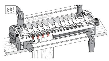
**12-6** At the back of the desk both sides and top are flush, so the rear edges are set against the side stops. Place the left end of the top tail board against the left side stop  $\P$ . Rout the tails.
