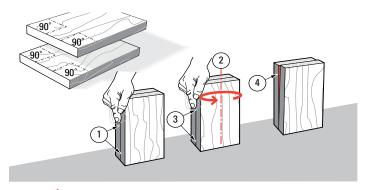
**6-2** Check for squareness: stand both pieces vertically on a flat surface. Make sure side edges are flush at bottom and top ①. Turn one piece around on its end ②. If side edges are flush top to bottom ③, the boards are square. If not, ④; cut two that are.
