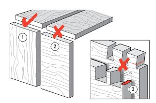
**6-3** Dovetail joints are intended for joining end-grain to end-grain ①. Attempting to rout dovetails in side grain ② will not work because:
