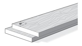
**6-4** You will want to test the jig, so prepare some 3/4" x 51/2" [20x140mm] boards. Cut them to length as you need them for the jig tests you want to perform. Use them for practice with the jig's various joint modes so you can see how the different modes work. Remember, though, that two boards of different thicknesses can be joined just as easily.
