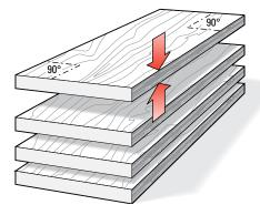
**6-1** It is vital for accurately aligned joints that stock used on the Superjig should be prepared straight, flat, of even thickness and equal widths, with square ends and edges. *Note that plywood is generally unsuitable for routing because of tearout problems.*
