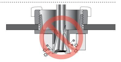
5-8 Never release the router plunge mechanism when using dovetail bits. Check if your plunge router has a stop nut to prevent this from happening accidentally.
