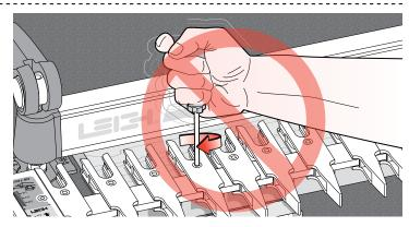
**2-4** Do not over-tighten the guidefinger lock screws. The Leigh screwdriver provided will give ample torque for easy lock-up without strain.
