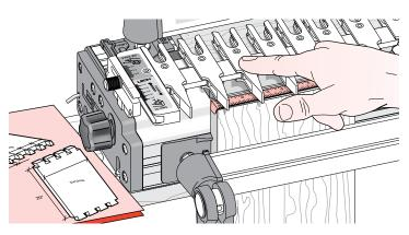
**2-6** You can adjust the guidefingers by eye, or by measurement to suit a set of plans.
