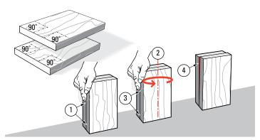
**1-7** Now you need two boards about  $\frac{3}{4}$ " x 6" x 8" long  $[20 \times 150 \times 200 \text{ mm}]$ . Both must have perfectly square ends to accurately index the front and rear side stops.
