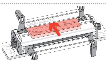
**1-12** Make up a  $\frac{3}{4}$ "x 6" [20 x 150mm] finger support board as shown. Lengths: 11" [280mm] for Super12, 17" [430mm] for Super18, and 23" [600mm] for Super24. Use MDF or plywood for flatness and stability. This board will support the guidefinger assembly in all front-clamping vertical board modes. Clamp it in the rear of the jig.
