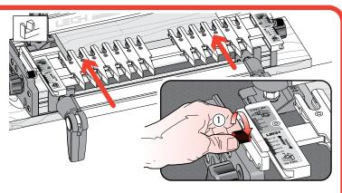
**1-14** Slide the finger assembly onto the support brackets, in the PTD Pin mode and set on the <sup>1</sup>/<sub>2</sub>"[12,7mm] setting. First, tighten both thumbscrews ①.
