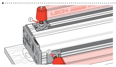
**1-5** Place four springs ① and two clamp bars on the T-bolts. Make sure the clamp bars move freely on the T-bolts.
