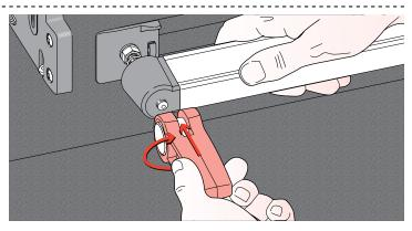
**1-6** Screw a clamp lever assembly onto each T-bolt.
