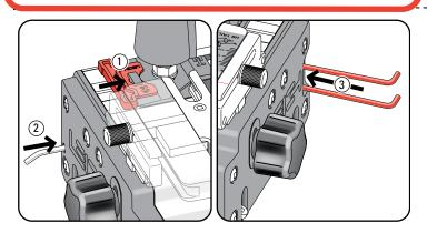
**1-17** Finally, slip the Spacer on the outside of the left rear side stop ①, the nylon stop rod through its storage hole in the left end ② and the pin wrench in its slot in the right hand end housing ③.
