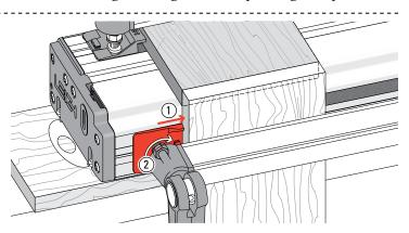
**1-10** Now push the front left side stop inwards and flush against the vertical board ① and firmly tighten the clamp bolt nut. **Repeat operations 1-8 thru 1-10 at the right side of the jig.** The front and rear side stops are now indexed to provide accurate board alignment in all routing procedures. You may now remove the boards.
