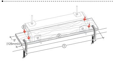
**1-3** Prepare a flat <sup>3</sup>/<sub>4</sub>"[20mm] mounting board (plywood or MDF), at least 5"[125mm] wide. Length ①: 26" for Super12, 32" for Super18, 40" for Super24 [660, 830 or 1000mm respectively]. Clamp it to the front of your bench. Center the jig on the board, front face slightly overhanging the board edge ②. Mark the four hold down screw positions. Drill small pilot holes at a slight angle ③.
