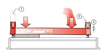
**1-21** For all but the wider workpieces, you need only operate the clamp on the workpiece end of the jig to release the board ①. For narrower boards, the clamp at the free end ② should be just tight enough to bow the clamp bar about  $\frac{1}{16}$ "[2mm] ③.
