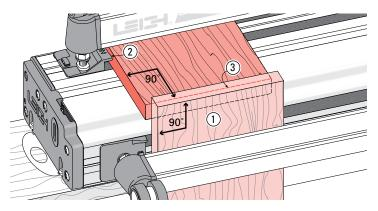
**1-8** Align Front Side Stops Clamp one square ended board in the front, not touching the left side stop and with the top edge above the top surface of the jig body ①. Place the other square board in the rear clamp, tight against the left rear side stop ②, with its front edge touching flush across the rear of the vertical board ③. Tighten the rear clamp. *Note: Do not overtighten the right hand clamps during this step.*
