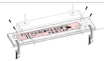
**1-4 Quick Reference Pull-Out** Decide which end of the jig you wish to access the "Quick Reference" instruction pull-out and place the jig over the pull-out ①. Using the screws provided; screw the jig to the board. Make sure that the pull-out slides freely.
