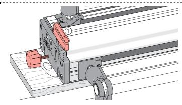
**1-11** Insert the right and left support brackets. Attach the knobs, raise them to full height and tighten the knobs.
