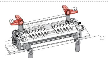
**1-22** When engaged, the front clamp levers should normally point down and the rear levers should point away from the operator ① or up to 90° either side ② as required to obtain the optimum clamping pressure.
