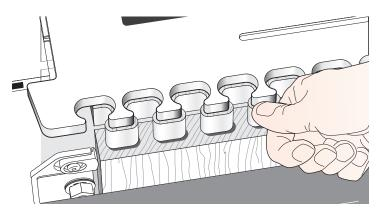
**11-10** Before removing the board, examine the routed sockets to ensure a clean cut.
