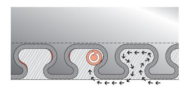
11-3 Go back from right to left to make a final cleaning cut and to ensure no tiny parts have been missed.
