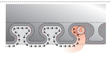
**11-2** Now rout left to right, following the template contours to rout out the pins.
