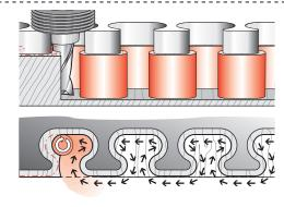
**11-7** Now rout right to left, following the template contours, the bit still set at 90% depth. Note: In thicker socket boards and hardwoods, rout in several passes at progressively deeper cuts.
