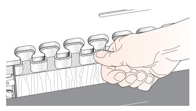
**11-4** Before removing the board, examine the routed pins to ensure a clean cut.
