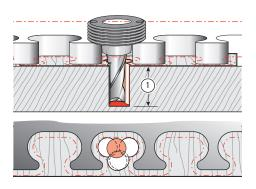
**11-6** The quickest solution in troublesome wood is to plunge two to four times in each opening to 90% of board thickness only ①.
