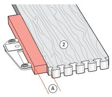
**7-2** Block drawer sides ② away from the side stops by one complete pattern pitch A.
