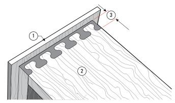
**7-1** Rabbeted drawer fronts ① and the mating sides ② have to be blocked away from the side stops. Dimension ③ must be minimum  $\frac{11}{16}$  [17,5mm].
