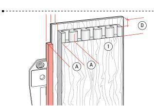
**7-3** Block the drawer front ① away from the side stop by B which is pattern pitch A minus rabbet width C. Adjust bit depth to D (rabbet plus drawer side thickness). ■
