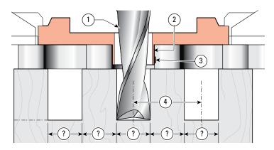
**4-2** If Isoloc joints were routed with nominal-size straight bits ① and nominal-size guidebushes ② against straight guide surfaces ③ on nominal pitch centres ④, there would be no possibility of guaranteeing a good fit. There are no angles to use for fit adjustment as there are with dovetails, so manufacturing tolerances for bits, guidebushes, templates and routers give an "average" fit which is rarely correct. *To illustrate, we have used a simple box joint in this series of drawings.*
