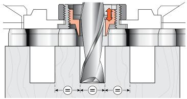
**4-6** A few trial-and-error test cuts and VGS adjustments will allow you to establish the right pin and socket sizes for a perfect fit. Note: One eighth of a turn of the variable bush changes the joint glue-line interface by one thousandth of an inch (.001"[.025mm]).
