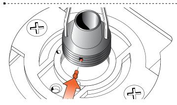
**4-7** Fit the holder to the router first. Before fitting a variable bush to a holder, fit a nylon thread insert in the hole in the thread. Leave the insert on its "tree" and push into the hole. Then snap off the "tree". The insert will become trapped and should not fall out when removed. However, if you remove the bush from its holder, wrap some scotch tape around the bush to prevent this. The spare inserts will last a long time.
