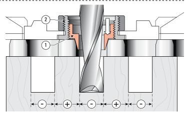
**4-4** With the VGS tapered bush ① screwed down in the holder (away from the router) ② the active bush diameter is increased, allowing no side-to-side movement, and resulting in smaller sockets and larger pins. A tight fit! *Guidebush angle, scale and movement are exaggerated in this sequence of illustrations.*
