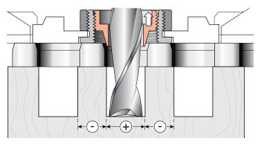
**4-5** Raising the bush (screwing the bush up into the holder) allows more side-to-side router/bit movement, producing larger sockets and smaller pins, and thus a loose fit. △ Do not rotate VGS more than three full turns above flush.
