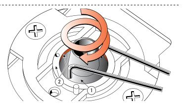
**4-8** Always start test routing with the bush flange ① turned one to one-and-a-half turns farther in than the holder flange ②.
