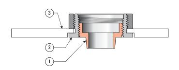
**4-3** The Leigh VGS bush has a tapered barrel ① threaded into a holder ② which in turn attaches to an adaptor or directly to the router ③.
