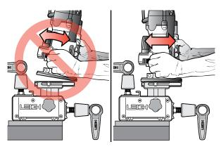
**2-5** Do not tilt the router on the jig. Keep the router flat on the jig assembly.
