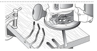
**2-8** If you have never used your router before, be sure to follow the router manufacturer's instructions for its use. Make plenty of simple open-face practice cuts *without a guidebush* before you try to use the router on the Leigh jig. You must, of course, always use a guidebush when routing on the Leigh Jig.
