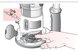
**2-4** Always disconnect the power source from the router when fitting bits or guidebushes, or making adjustments.
