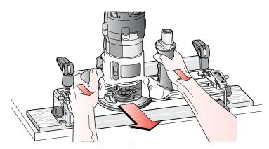
**2-6** If you insist on removing the router from the jig while it is still revolving, always pull it straight off the jig horizontally, and do not raise or lower the router until it is completely clear of the jig.
