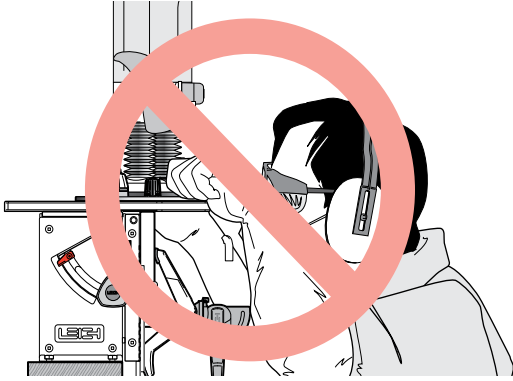
3-46 Do not rout at face level.
