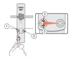
**A2-8** The sidestop fence is squared at the factory, but check your first test joints. If your router/bit is not perfectly perpendicular to the table adjust the sidestop fence: slightly loosen the 'pivot' screw ① and the 'lock' screw ②. Adjust the angle ③ to match the bit and retighten. Rout test joints to confirm correct setting. Once locked in this position it should never need adjusting when used with that same router.
