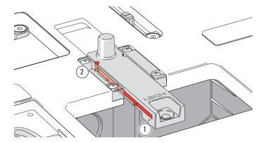
**A2-7 Jig Maintenance** Very little maintenance is required. Fine dust build-up in the front and rear sight stops should be removed from time to time. The end of the small hex key or a piece of wire will do the trick. At the front ① and with the sight to the rear position at ②. Dusting off with compressed air (if available) will keep the jig clean.
