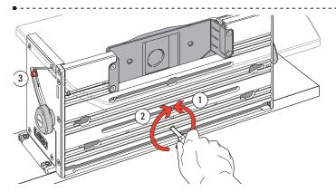
**A2-3** The adjusting screw for setting the clamp plate is in the lower center of the plate. Loosen the quadrant knobs. Use the hex screwdriver to turn the screw counterclockwise to move the plate in ①. Turn the screw clockwise to move the plate out ②. The screw is treated with Loctite<sup>TM</sup> to prevent accidental rotation. When the clamp plate is square, re-zero the angle indicator if necessary ③.
