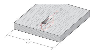
A1-12 Maximum Width Mortise Board for Mortising to Center Width from 45/8"[115mm] up to 6½"[165mm] ①. See 6-22 for special instructions. ■
