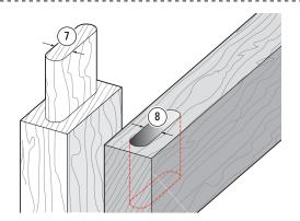
A1-3 Thick or thin tenons ⑦ fit into wide or narrow mortises ⑧.
